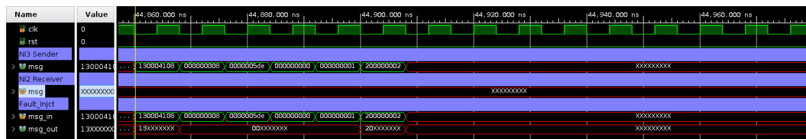
Figure 7.14: Illustration of messages exchanged between NI3 and NI2, without redundancy mechanism, fault is activated
