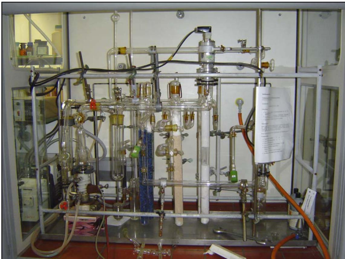
**Fig. 3.2:** Photo of the vacuum manifold used for ampoule evacuation
