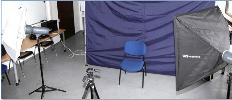
Figure 3.4: A DSLR camera mounted on the tripod in the foreground and two external flash units are used to capture high resolution images of a person under controlled lighting conditions. This guarantees uniform illumination of each face. Later, these photos are used to extract a high quality texture which is mapped onto the scanned 3D shape of the corresponding person.
