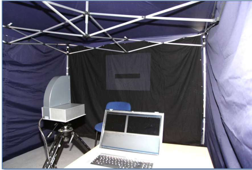
Figure 3.5: The structured light scanner projects a sequence of parallel lines that vary in width onto the face of a person (see Figure 3.6) and captures these 2D images. The patterns of these projected lines in the series of 2D images are used to estimate the 3D shape of the face. With this scanner it is possible to capture detailed 3D information but stray light of the environment may lead to artifacts in the scans. Therefore, the capturing process takes place in a dimmed environment inside a dark tent.
