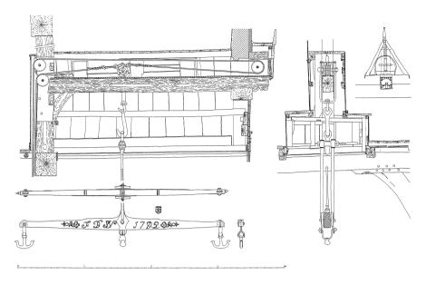
93 Trolley with scale in the so-called Enkhuizen weigh house, measured drawing
