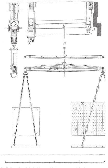
92 Trolley with scale in the Hoorn weigh house, measured drawing
