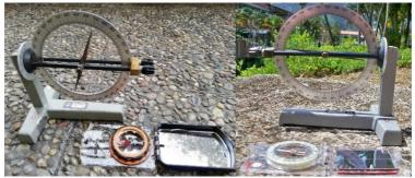
*Fig. 4: The use of an inclinatorium in Siegen (left) and Quito (right): Clearly observable is the difference of inclination. Photo: Volker Heck.*
