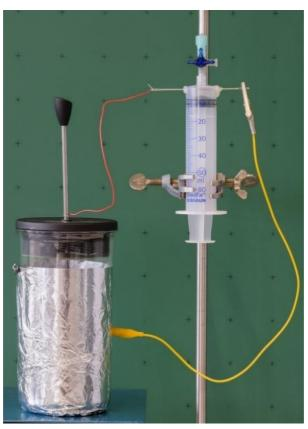
Figure 1: Oxyhydrogen gas eudiometer to determine the oxygen content of air by reaction with hydrogen
