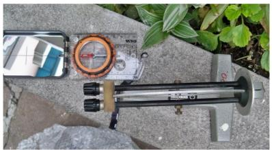
*Fig. 3: Measurement setup to determine the inclination in one place. The parallelism of the inclinatorium and the connecting line of the magnetic poles is important. Photo: Volker Heck.*
