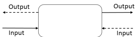
Figure 8.1: Input and output ports of a tile in a double ring architecture.
