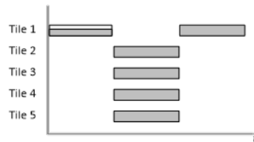
Figure 5.2: Local energy management: When the execution is faster than the schedule's WCET, the tile can locally perform DVFS and lower the execution frequency to finish at the expected WCET avoiding idle times in the scheduled time
