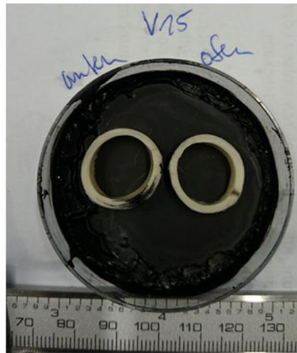
Figure 4-3 Ring-shaped cross sections of the porcine aortic specimen for optical measurement of its load-free wall thickness. Handwritten notes give the sample number (“V15”) and identify the longitudinal position of the sample from which the two rings were cut (“unten”, “oben”). [Image: C. Blase, Cell and Vascular Mechanics Group, Goethe University Frankfurt.]
