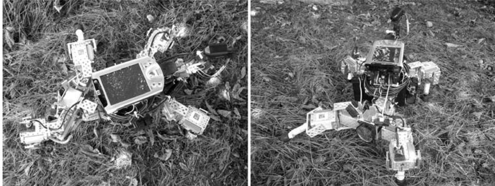
Figure A.1: The physical four-legged walking machine AMOS-WD02. Left: Top view with turning its backbone joint. Right: Front view with standing position.
