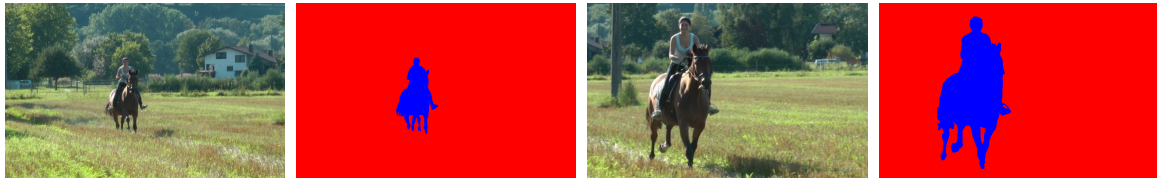
Fig. 2.7 Motion segmentation example is provided for frames 1 and 160 of the “horses01” sequence (with their ground-truth motion segmentation) in the FBMS59 [123] dataset. Due to the reason that the person and the horse move together and have the same motion pattern, the same motion label (blue color) is assigned.
