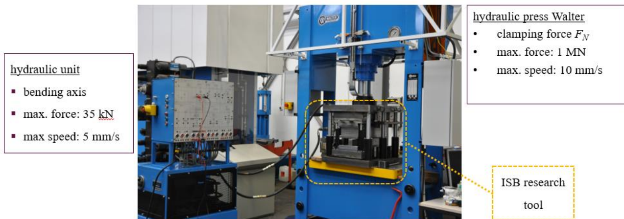
Figure 46: WALTER WUP press with independent hydraulic unit attached to the ISB research tool.
