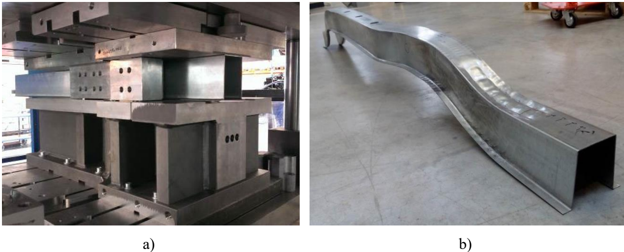
Figure 100: Industrial demonstrator production in the R&D project “ISB-ELEKTRO” according to STÖTZEL (2017). ISB industrial scale tool (a) equipped on the SCHULER MSE 2-1000-3.5-600 press for ISB manufacturing of continuous longitudinal members (b) for the substructure of an electric vehicle. The component features two bending planes (lateral and vertical in relation to the cross section) which are realized by individual tool inserts.
