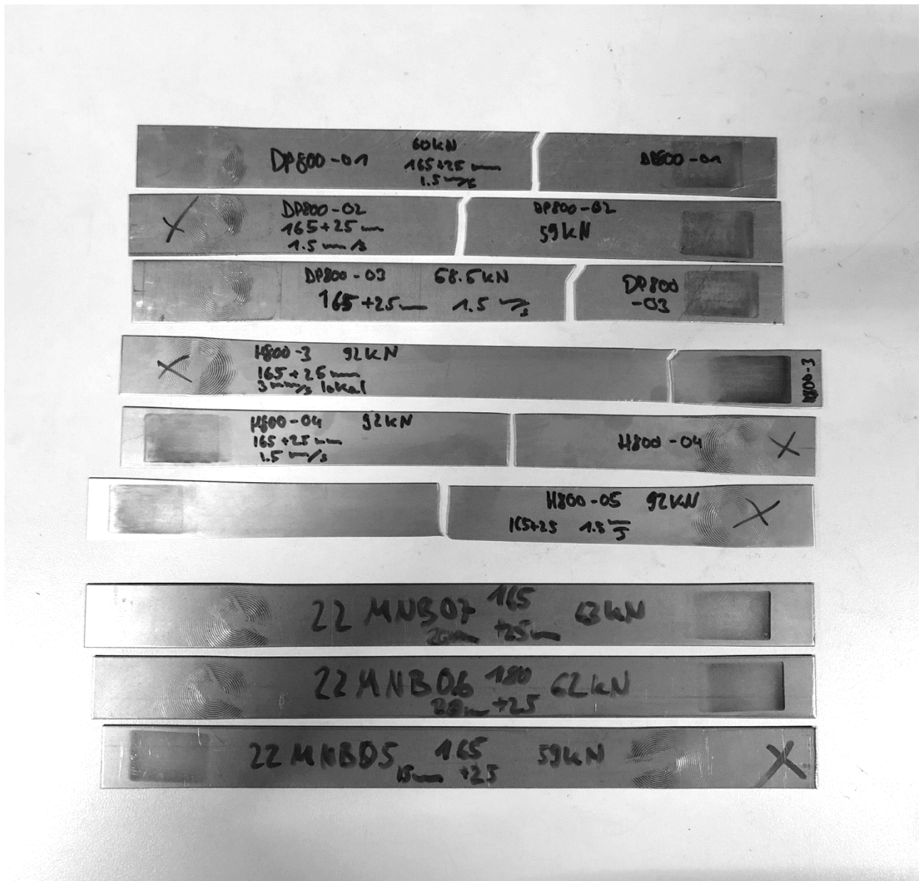
Figure 121: Strips from HCT780X, Forta H800 and 22MnB5 tested under plastic tensile deformation in strip drawing.
