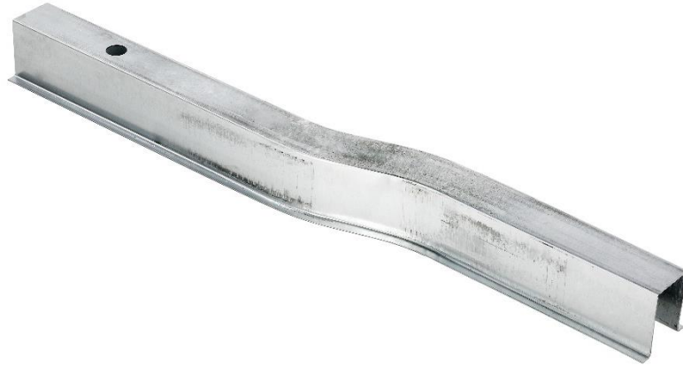
Figure 83: Bending geometry of the use-case considered for systematical process layout.
