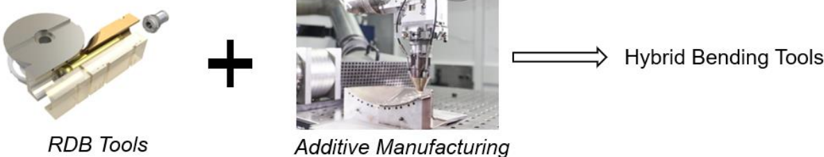
Fig. 5: Concept of manufacturing hybrid bending tools
