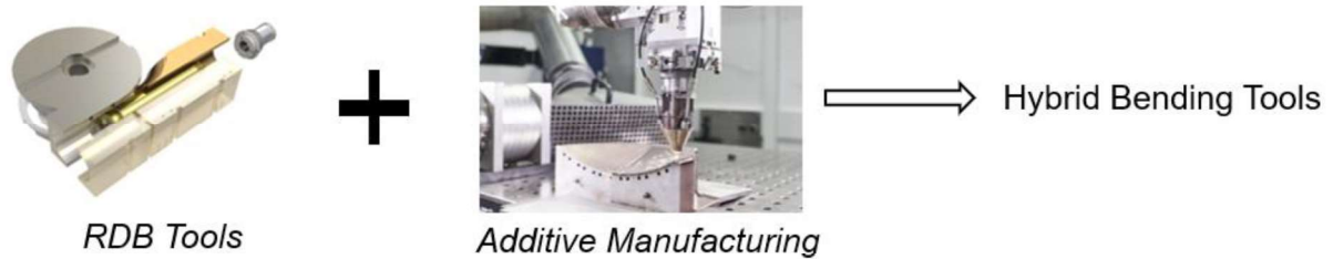
Fig. 5: Concept of manufacturing hybrid bending tools
