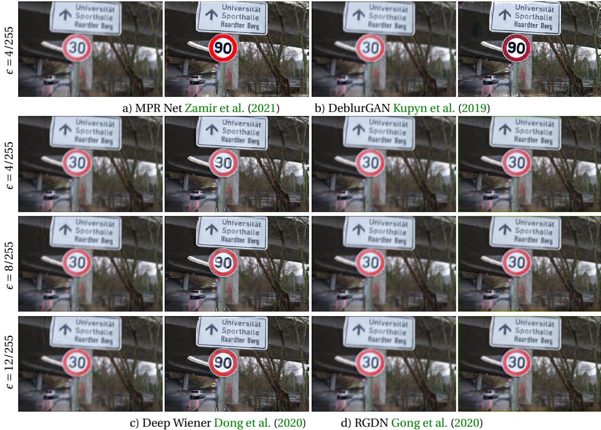
Figure 6.4: Illustration of localized targeted attack. For each approach, the first column is the adversarial input and the second column is the network prediction.
