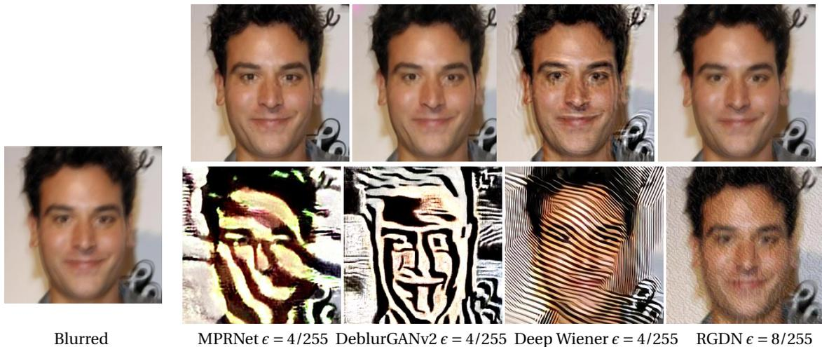
Figure 6.5: Untargeted adversarial attack on deblurring networks MPRNet [Zamir et al. \(2021\)](#), DeblurGANv2 [Kupyn et al. \(2019\)](#), Deep Wiener [Dong et al. \(2020\)](#), RGDN [Gong et al. \(2020\)](#). Blur kernel ‘6’ of size  $21 \times 21$  in the dataset of [Sun et al. \(2013\)](#) is used.
