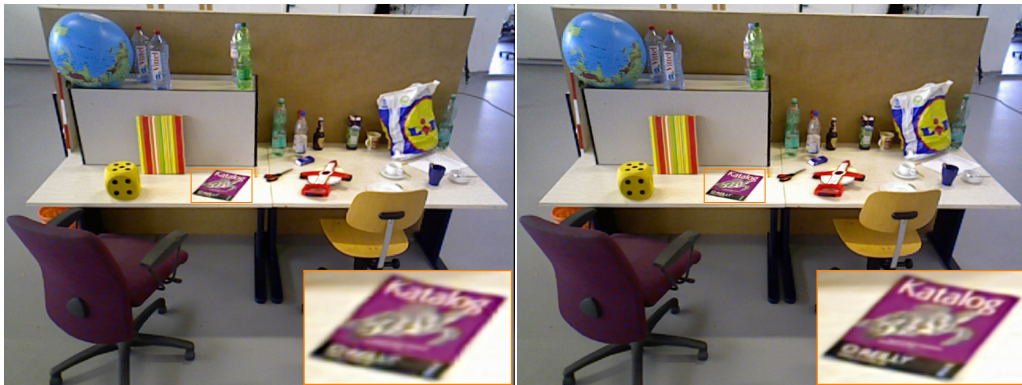
Figure 4.16: Robustness against self-localization drift. Refinement of the LongOfficeHousehold data set before exiting the reference viewpoint (left) and the final refinement after re-entering the reference viewpoint (right) using the presented approach. See also Figure 4.7 for a comparison with the unrefined reference image.
