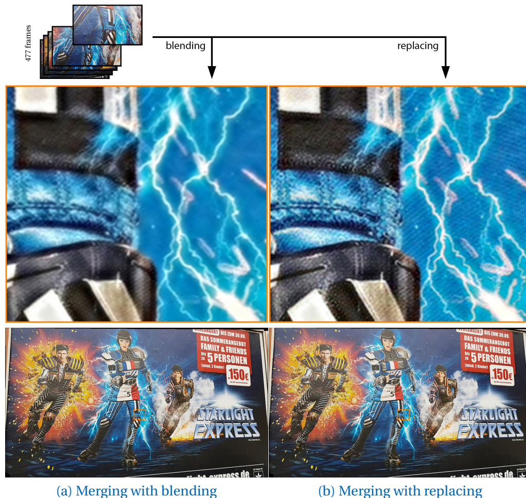
Figure 3.15: Starlight (477 frames): Comparison between a blending using cumulative average weighting (left) and the described replacement strategy (right) applied to a 477 frames sequence captured with a Samsung Galaxy S8 built-in camera.
