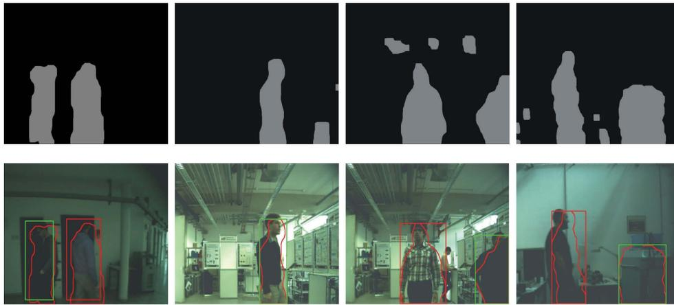
Figure 4.6: Top: Foreground images derived using background subtraction technique. Bottom: Corresponding 2D images with detected contours as object of interest. It is noticeable that due to the low resolution of 3D images, the contours which are derived from range data do not completely fit to the boundary of their corresponding objects in the 2D images.
