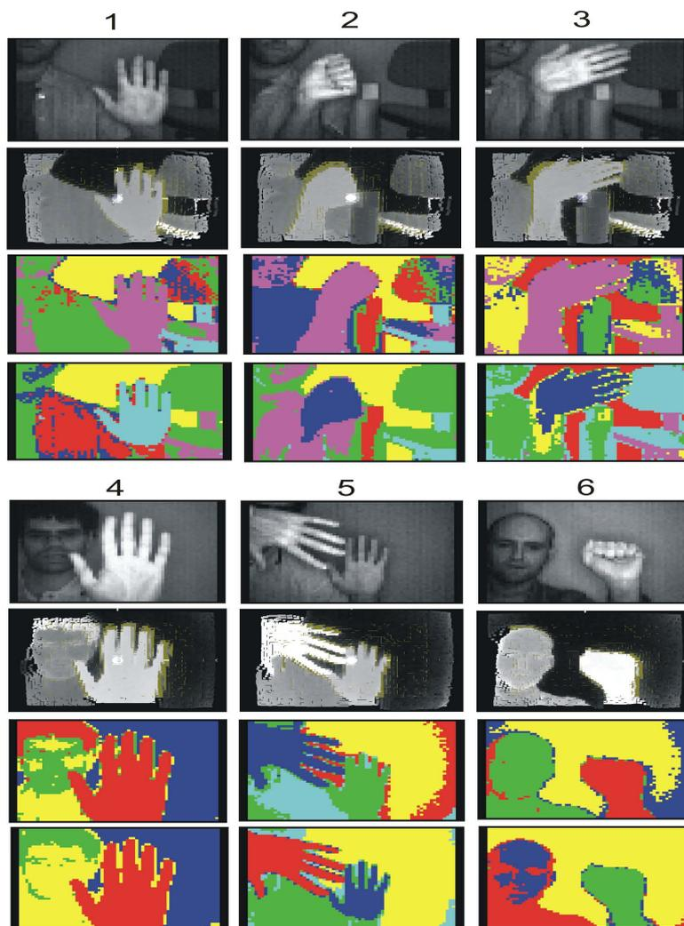
Figure 3.17: Results of hand gesture segmentation in a complex scene. First row: Intensity images. Second row: Range images. Third row: Segmented images using range feature. Fourth row: Segmented images using the fusion of range and phase features [50].
