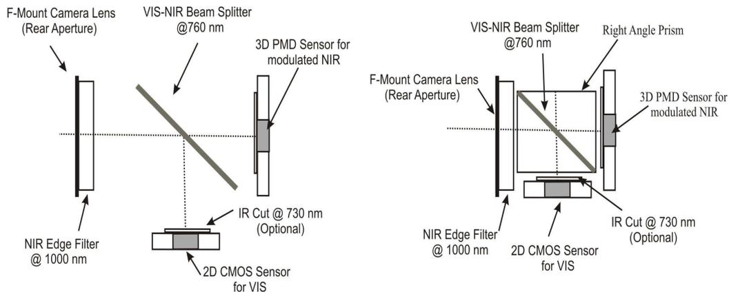
Figure 2.5: Optical setup of the MultiCam. Left: F-mount, Right: C-mount [12], [35].
