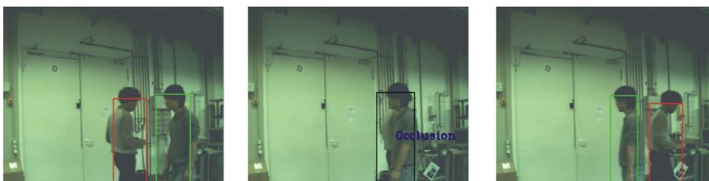
Figure 4.12: Occlusion handling. Left: Before occlusion. Middle: Occlusion detected and labeled. Right: After occlusion.
