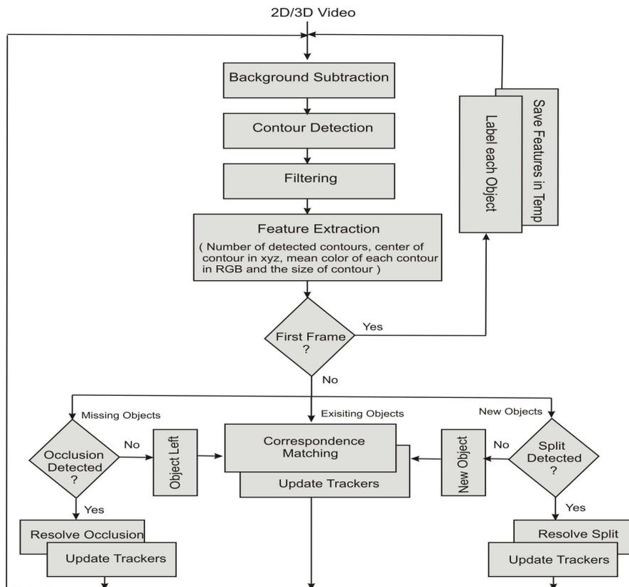
Figure 4.7: Flowchart of feature extraction and correspondence matching technique.
