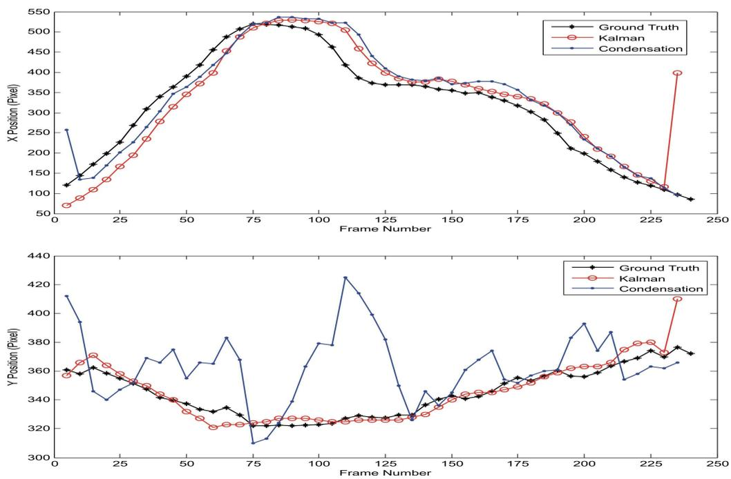
Figure 4.16: Trajectory of the person in the image coordinate system. Black: Ground truth, Red: Kalman filter, Blue: CONDENSATION. Top: Trajectory in x direction. Bottom: Trajectory in y direction.
