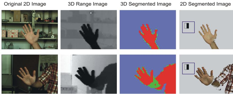
Figure 3.31: Solution to the background issue in object detection using the Viola-Jones method. Using range data, the cluttered background is removed and the foreground image is segmented and mapped to the 2D image. The Viola-Jones technique is applied to the 2D segmented image to find the object of interest.
