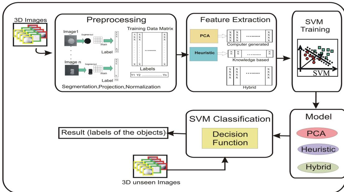
Figure 3.26: Flow of the moving object classification algorithm.
