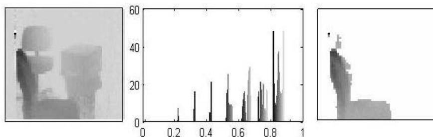
*Figure 3.13: Range Segmentation. Left: TOF range image subtracted from the background. Middle: Normalized histogram of range image. Right: Range segmented object.*
