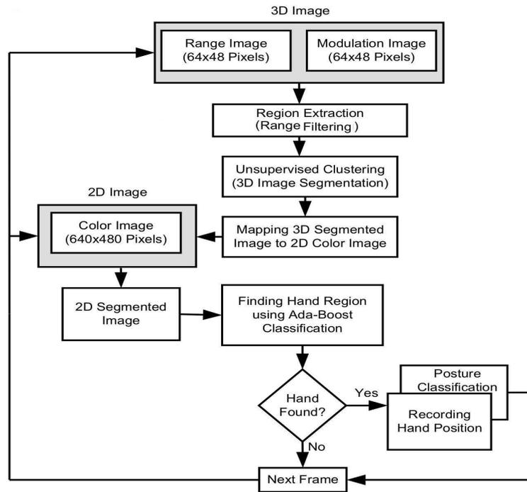
Figure 4.13: Block diagram of the hand detection algorithm.
