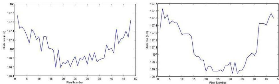
Figure 2.6: Left: Range measurement before filtering. Right: Range measurement after filtering.
