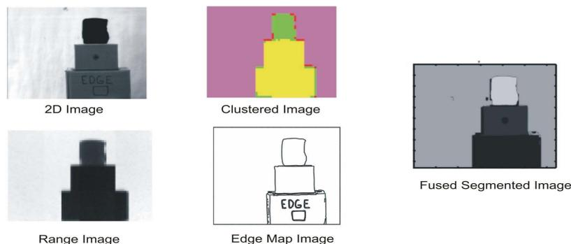
Figure 3.23: Object segmentation using the integration of clustering and edge detection - complicated case with texture.
