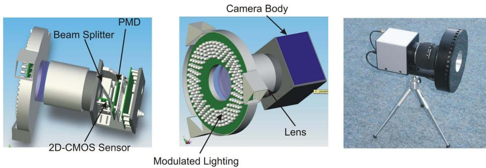
Figure 2.4: The MultiCam 2D/3D vision system developed at ZESS.
