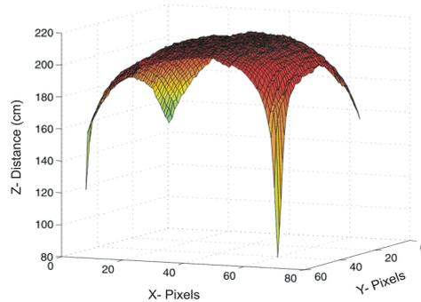
Figure 2.8: Out-of-range errors appear in the corners of a plain surface which are out of the illumination zone of the lighting system.
