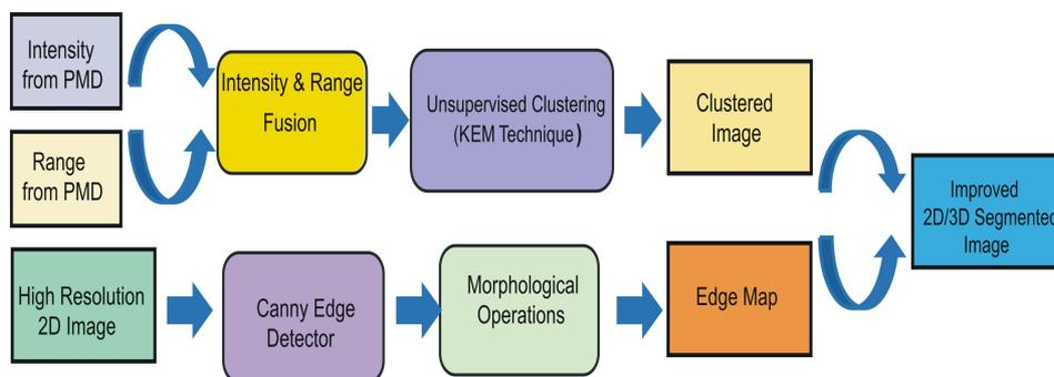
Figure 3.21: Block diagram of the improved segmentation technique.
