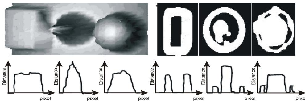
Figure 3.27: Range images of the multi object set including box, ball and cone. Top Left: TOF range images. Top Right: The stereo range images and the lower row shows the longitudinal sections through the middle of each range image.
