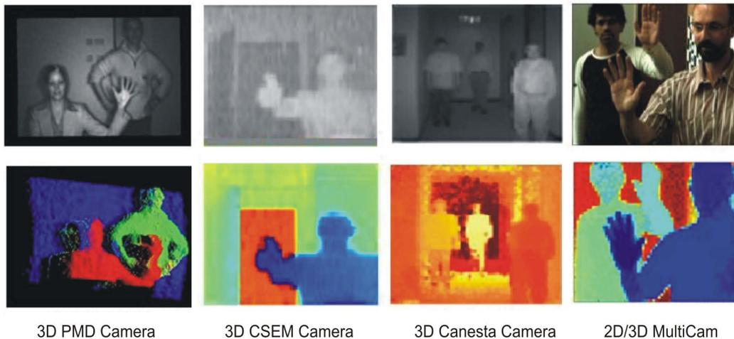
Figure 2.3: Some Time of Flight 2D/3D images. First three columns: Low resolution intensity and range images taken by three different TOF cameras: PMD [31], SwissRanger [29] and Canesta [28] respectively. Last column: 2D/3D image taken by the MultiCam.
