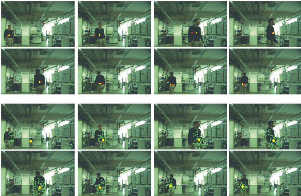
Figure 4.15: Some results of person tracking using the Kalman filter and the CONDENSATION technique (frame number 10, 35, 60, 150, 185, 215, 225, 235). First two rows represent the Kalman filter results. Red point shows the predicted (intermediate) position and yellow shows the corrected point (final result). Last two rows represent the CONDENSATION result where the particles are depicted in green and the mean of all (final result) is in yellow.
