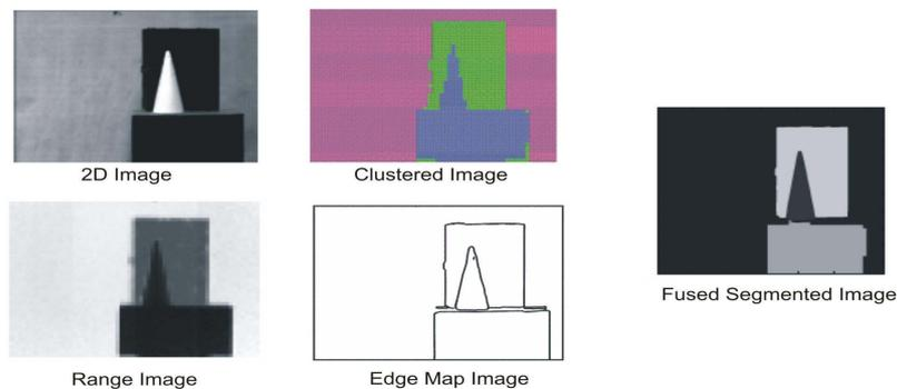
Figure 3.22: Object segmentation using the integration of clustering and edge detection - simple case.
