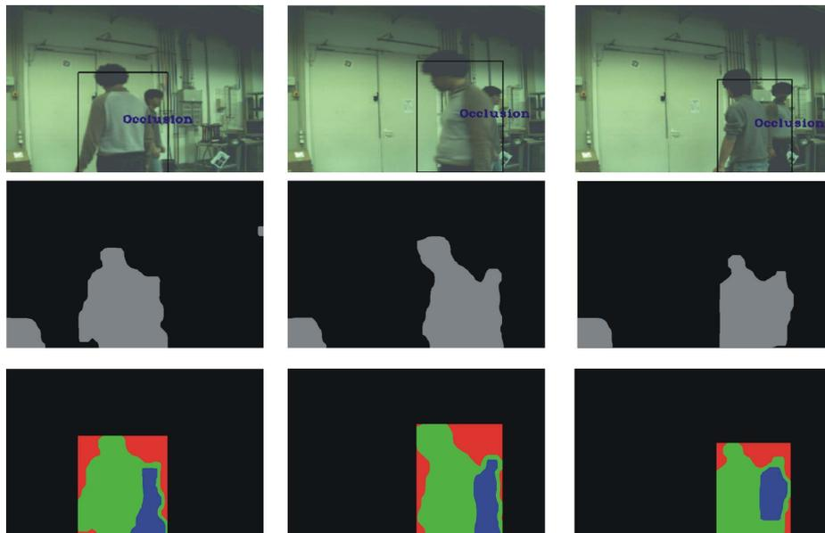
Figure 4.10: Segmentation of merged objects during partial occlusion using range data and based on the K-means clustering technique. Top: 2D images, occlusion has been detected and labeled. Middle: Foreground range images. Bottom: Segmentation of merged objects.
