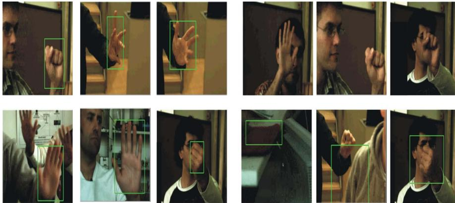
Figure 4.14: Some results of hand detection. Left: Example of correctly detected images (True Positive). Right: Example of wrongly detected images (First row: missed hand - False Negative. Second row: misclassified-False Positive).
