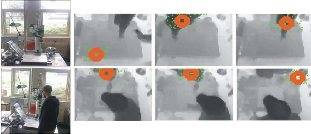
*Figure 5.4: Tracking of robot in the workspace using range images. The presence of the human in the safe zone does not confuse tracking. First column: Images taken by a normal camera from the scene. Last three columns: Robot tracked in 3D range images, green points are the particles and orange circle represents the center of all particles.*
