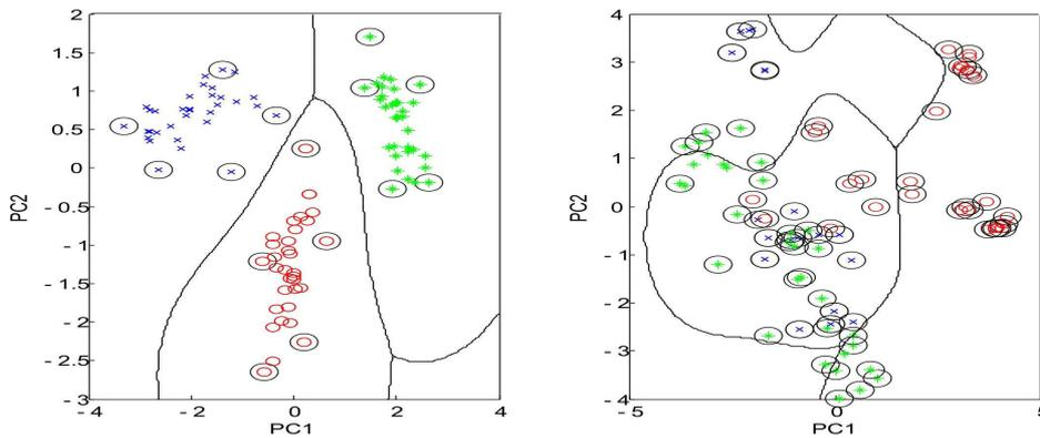
Figure 3.28: Distribution of the features on the first two principal components with the separating SVM based hyperplane. Left: TOF. Right: Stereo 1 (The support vectors are indicated by circles).
