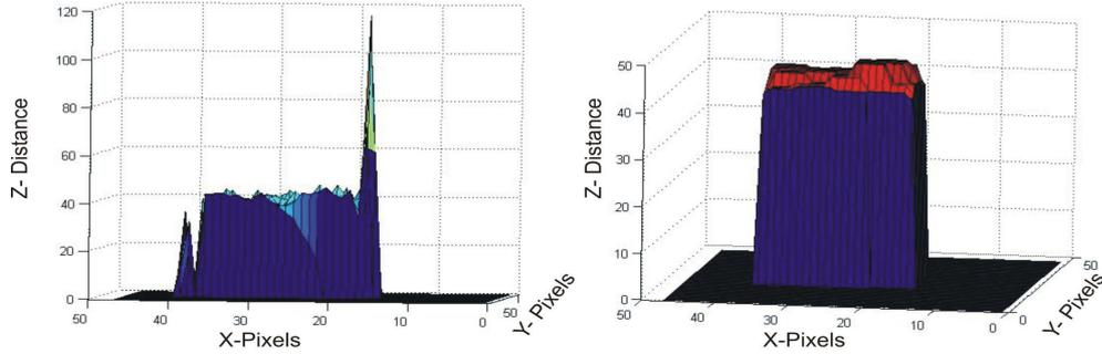
Figure 2.7: Left: 3D image from a box with motion artifact on the edges . Right: Motion artifacts are eliminated by morphological operations.
