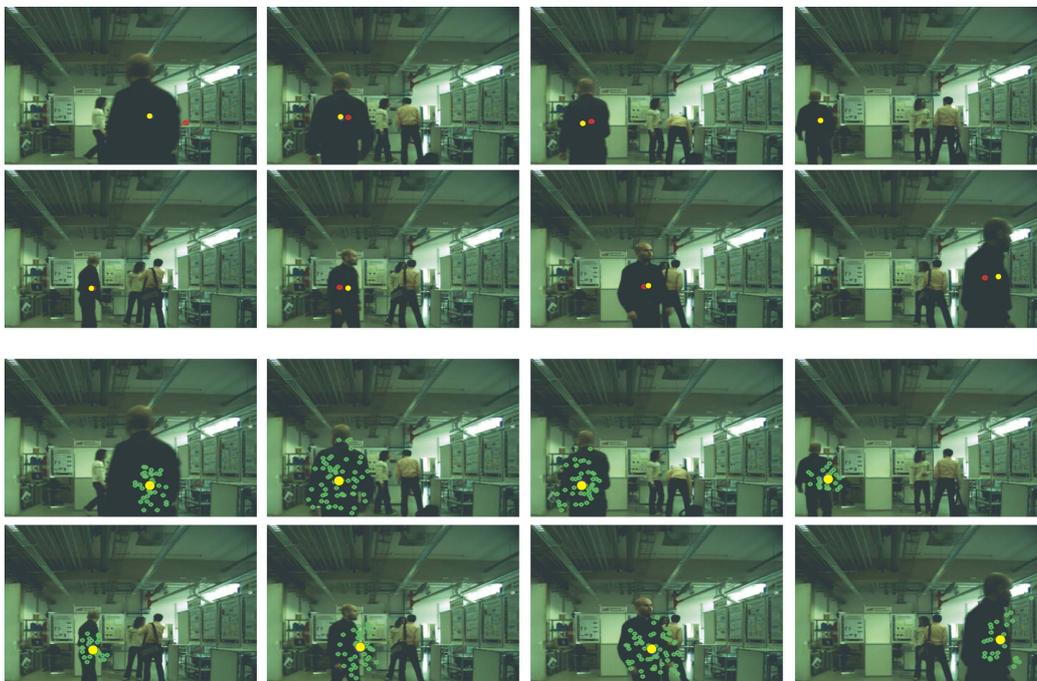
*Figure 4.17: Some results of person tracking using the Kalman filter and the CONDENSATION technique (frame number 55, 80, 95, 150, 195, 215, 275, 295). First two rows represent the Kalman filter results. Red point shows the predicted (intermediate) position and yellow shows the corrected point (final result). Last two rows represent the CONDENSATION result where the particles are depicted in green and the mean of all (final result) is in yellow.*
