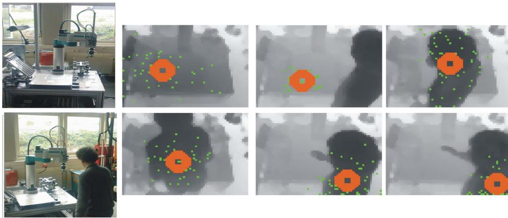
*Figure 5.5: Tracking of human in the workspace using range images and without presence of the robot. First column: Images taken by a normal camera from the scene. Last three columns: Human tracked in 3D range images, green points are the particles and orange circle represents the center of all particles.*
