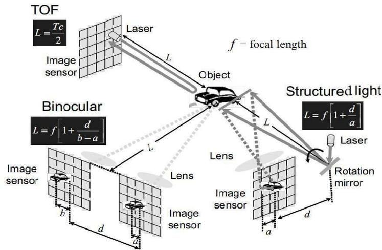
Figure 2.1: Conceptual schematic of some typical 3D range measurement techniques [4].
