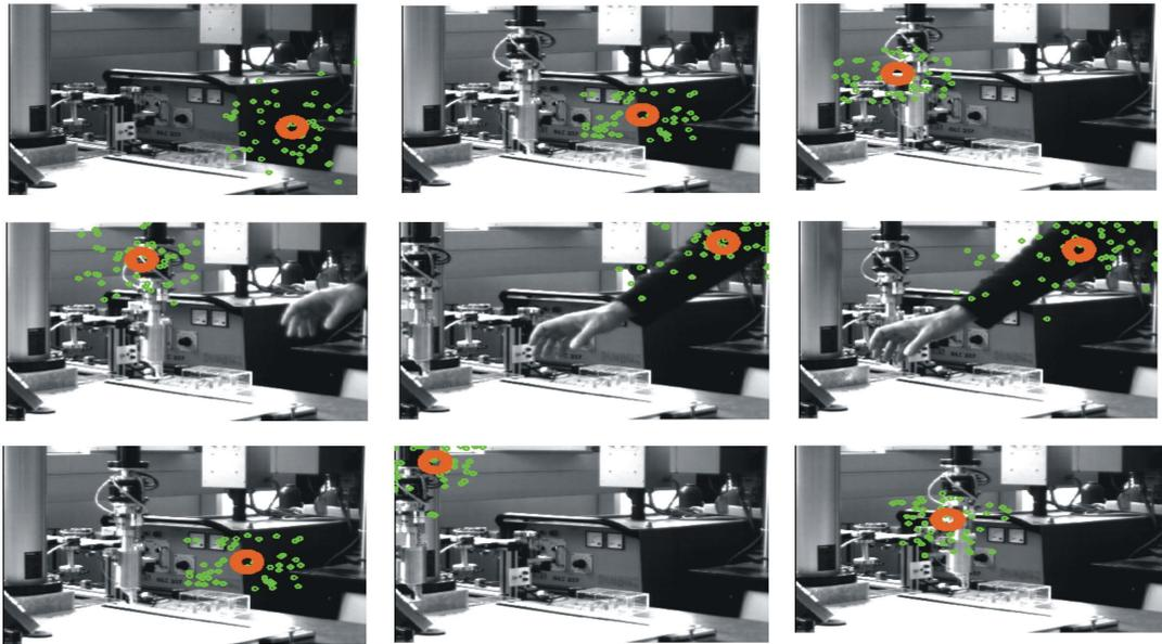
Figure 5.6: Tracking of the robot and the hand of an operator in the shared workspace using 2D/3D images, green points are particles and orange circle represents the center of the particle (final detected point).
