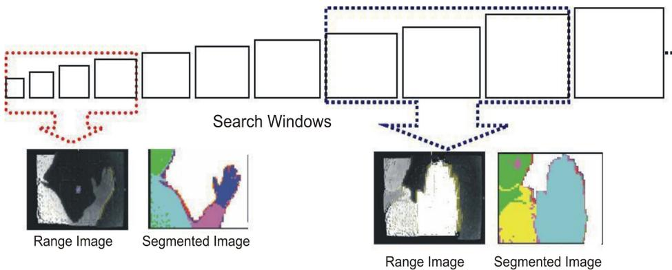
Figure 3.32: Selection of search windows using range information for hand detection. Left: Hand is far from the camera and therefore the image is searched with small search windows. Right: Hand is close to the camera and therefore the image is scanned with large search windows to find the hand in the image.
