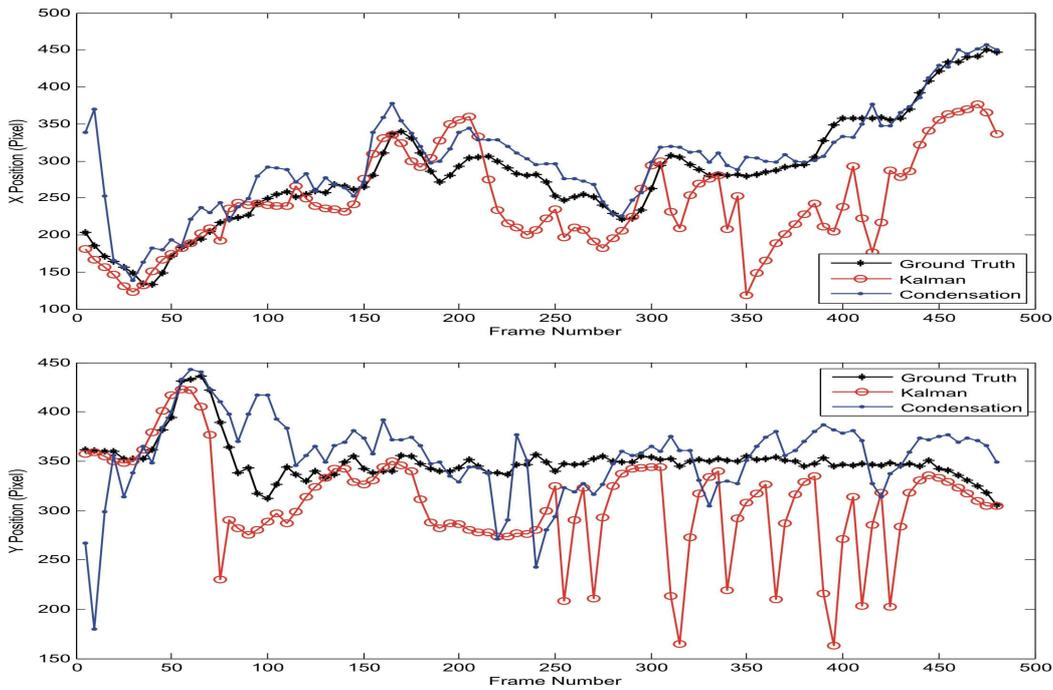
Figure 4.20: Trajectory of the person in the image coordinate system. Black: Ground truth, Red: Kalman filter, Blue: CONDENSATION. Top: Trajectory in  $x$  direction. Bottom: Trajectory in  $y$  direction.
