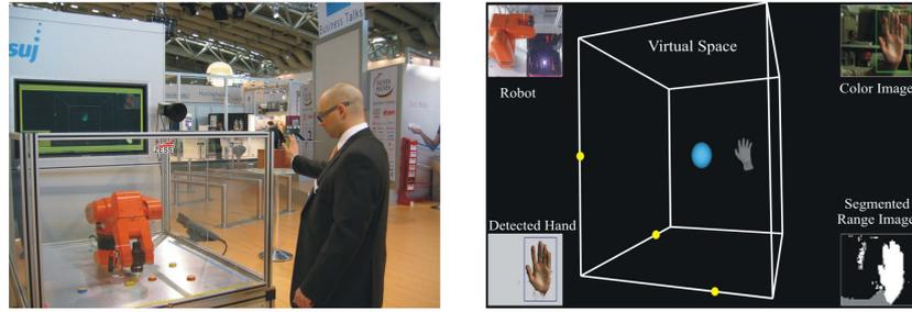
Figure 5.7: Left: Hand based robot control using Multicam, Hannover Fair 2008. Right: Graphical User Interface (GUI).
