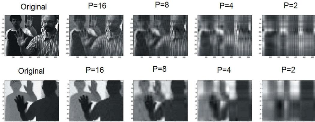
Figure 3.8: An example of image reconstruction. First row: The original 2D image together with its PCA reconstruction. Second row: The original range image together with its PCA reconstruction.
