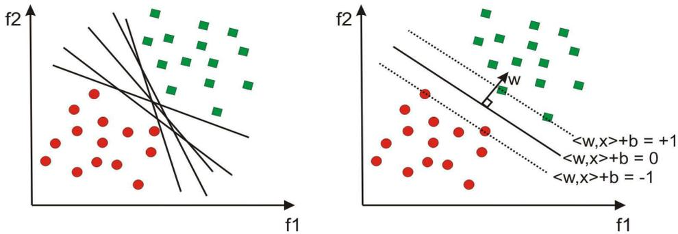
Figure 3.24: Left: Set of separating hyperplanes. Right: Optimal Separating Hyperplane (OSH). The dashed lines identify the margin.  $f_1$  and  $f_2$  represent two arbitrary features.
