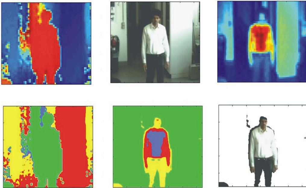
Figure 3.20: Human segmentation in 2D/3D images. Top Left: Low resolution range image from TOF sensor. Top Middle: High resolution 2D image. Top Right: Modulation amplitude image. Bottom Left: 3D rescaled segmented image. Bottom Middle: Rescaled segmented image using fusion of range and modulation amplitude data. Bottom Right: 2D segmented image result from mapping.
