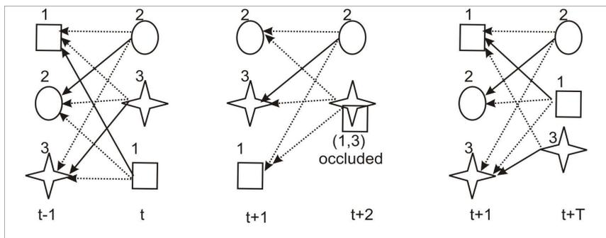
Figure 4.11: Correspondence matching. Left: Existing objects ( $n = m$ ). Middle: Object occlusion ( $n < m$ ). Right: Object split ( $n > m$ ). Note that after two objects split in frame  $t+T$ , they are matched to the objects before occlusion in frame  $t+1$ .
