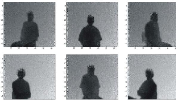
Figure 3.4: Some examples of range images from the person data set taken by MultiCam. The range data have been coded in gray values such that the darker the pixel, the smaller the distance to the camera.
