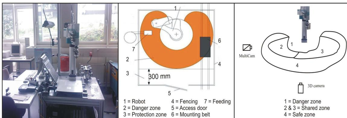
Figure 5.3: Left: Turboscara SR6, 4-axis robot which is used for our experiments. Middle: Space secured according to EN 775 given by the robot provider. Right: Dynamic safety system using MultiCam and 3D-PMD. The zones can be defined dynamically.
