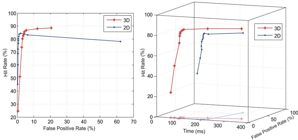
Figure 4.2: ROC curves for the image sequences under normal lighting conditions. Left: Trade-off between hit rate and false positive rate. Adaptive Gaussian mixture model using 2D images outperforms 3D range background subtraction. Right: Time dependent ROC curve. Considering time as the third evaluation parameter, 3D background subtraction outperforms 2D background subtraction.
