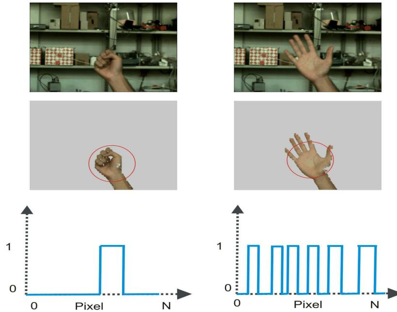
Figure 3.11: Knowledge based feature extraction using heuristics for hand pose classification. First row: 2D images. Second row: Hand detected images from 2D/3D data. Third row: The binary intersection function derived from tracing the circle.
