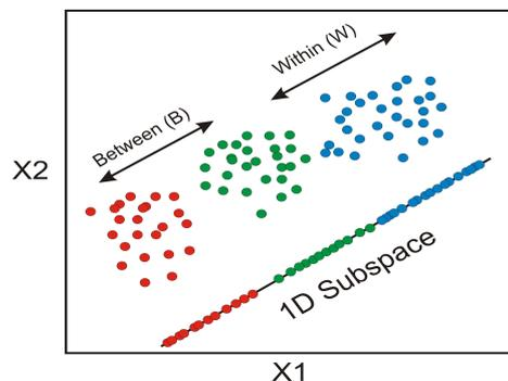
Figure 3.9: Projection of the 3-class feature data to a 1D subspace using LDA.  $X_1$  and  $X_2$  represent two arbitrary features.
