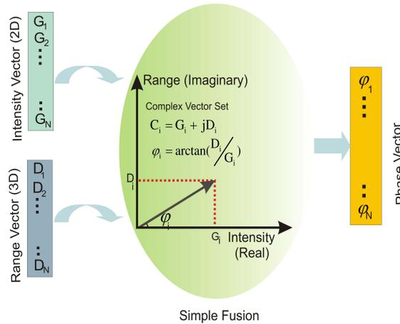
Figure 3.15: Flow of the range and intensity fusion.
