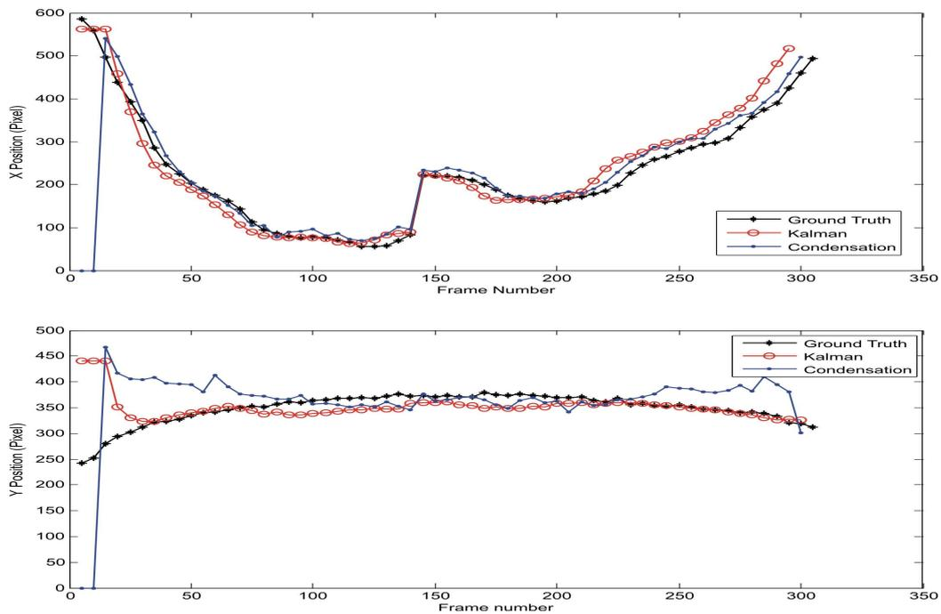
Figure 4.18: Trajectory of the person in the image coordinate system. Black: Ground truth, Red: Kalman filter, Blue: CONDENSATION. Top: Trajectory in x direction. Bottom: Trajectory in y direction.
