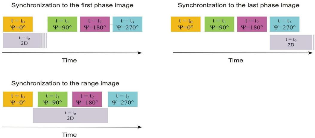
Figure 2.10: Different possibilities of 2D/3D Synchronizing in the MultiCam [12].
