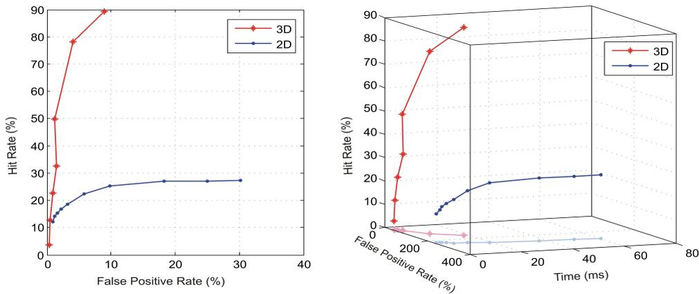
Figure 4.4: ROC curves for image sequences under varying lighting conditions. Left: Trade-off between hit and false positive rates. Right: ROC curve dependent on time. In both cases range thresholding followed by connected components outperforms the adaptive Gaussian mixture model using 2D images.
