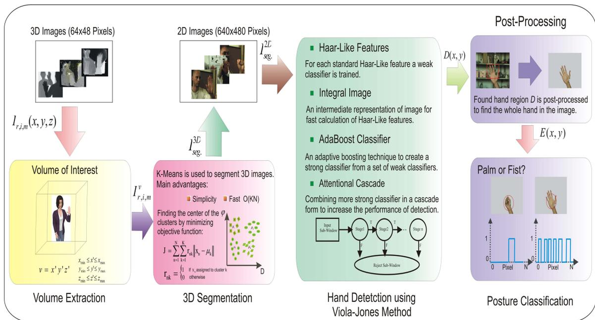
Figure 5.8: Hand detection and posture classification techniques for Hactor application.
