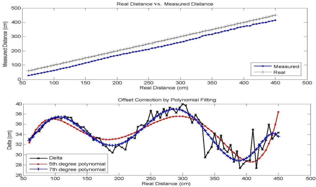
Figure 2.9: Range calibration. Top: Real distance versus measured distance. Bottom: Offset fitting and correction using polynomials.
