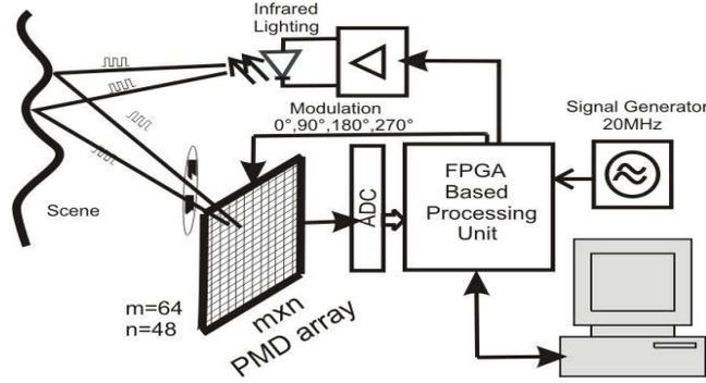
Figure 2.2: Conceptual schematic of ZESS-TOF camera based on PMD-3KS.
