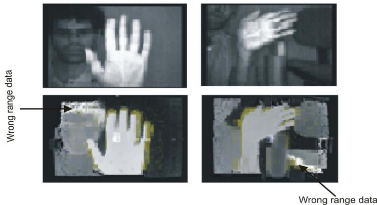
Figure 3.14: Two examples of TOF range mis-measurements. First row: TOF intensity images ( $64 \times 48$  pixels). Second row: Corresponding range images coded in gray values. Left: The hair gets wrong range data because of its black color. Right: The metal part of the chair has wrong distance data.
