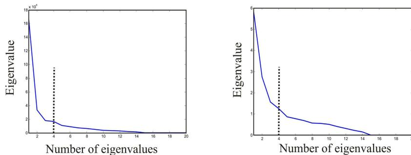
Figure 3.7: Eigenvalue spectrum, Left: Derived from range images. Right: Derived from 2D images. The first four eigenvalues have the highest slope.
