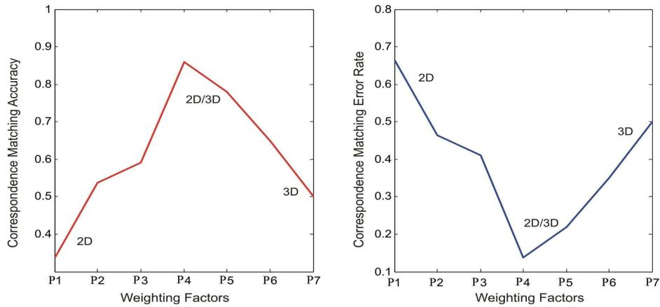
Figure 4.8: Performance of the correspondence matching technique over different weighting factors ( $P$  sets).  $P_1$  represents the weighting factor set where just 2D features contribute in making the similarity-based probability.  $P_4$  contains the weighting factors, where 2D/3D features contribute to the correspondence matching and  $P_7$  represents the weighting factor set where 3D features contribute in making the similarity-based probability.
