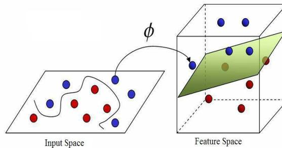
*Figure 3.25: Mapping the nonlinear input training data into a higher dimensional feature space via map function  $\phi$  [23].*
