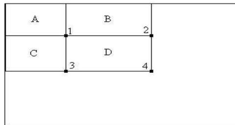
Figure 3.29: The sum of the pixels in the rectangle D can be calculated simply as:  $D=(4+1)-(2+3)$  where  $1=A$ ,  $2=A+B$ ,  $3=A+C$  and  $4=A+B+C+D$  [80].
