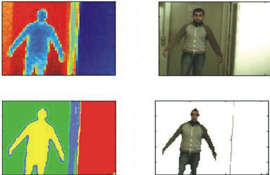
Figure 3.19: Human segmentation in 2D/3D images. Top Left: Low resolution range image from PMD-3K camera. Top Right: High resolution ( $640 \times 480$ ) 2D color image. Bottom Left: 3D segmented image using K-means and rescaled in high resolution. Bottom Right: 2D segmented image result from mapping.
