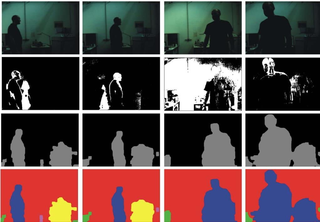
Figure 4.3: Some results of background subtraction under varying lighting conditions. First row: Original 2D images, frames number 130, 180, 310 and 415. Second row: Corresponding foreground images using the adaptive Gaussian mixture model on 2D images. Third row: Corresponding foreground images using range thresholding. Forth row: Connected components on 3D foreground images.
