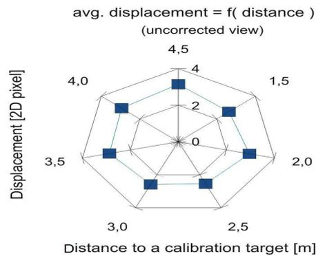
Figure 2.11: Uncorrected dislocation of PMD and 2D sensor in the MultiCam [12].
