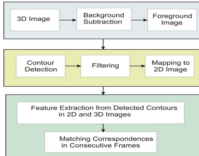
Figure 4.5: Block diagram of bottom-up tracking approach in general.
