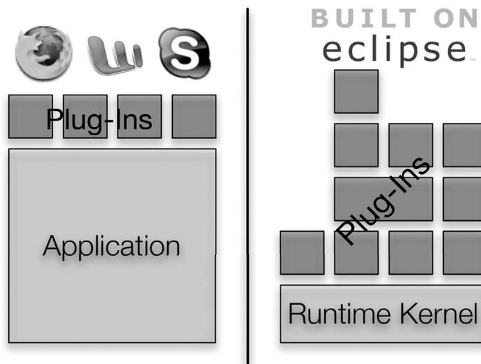
Figure 11: Architectures of traditional software (left) and the „every-thing is a plug-in“-approach of Eclipse (right) as perceived by it’s users.
