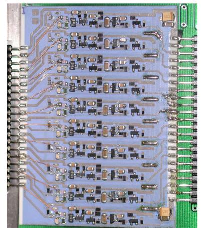
**Fig. 5.4:** 10-channel hybrid preamplifier
