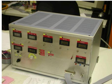
**Fig. C.13:** The power supply of the SDD
