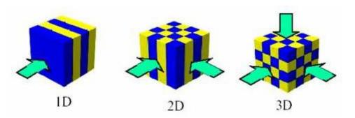
Fig. 1.1 1D, 2D and 3D phononic crystals [1]. (The arrows indicate the wave propagation directions).
