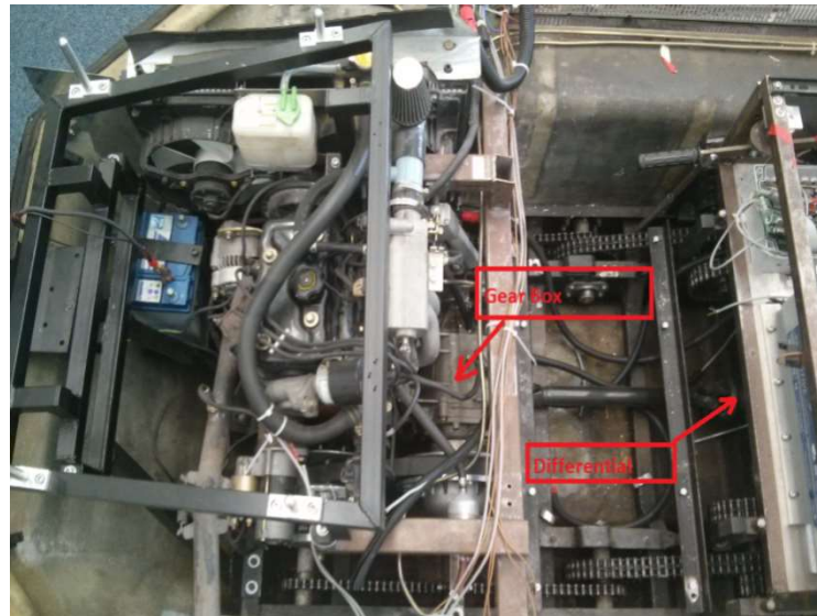
Figure 2.8 Mechanical driveline of Amphibious Vehicle
