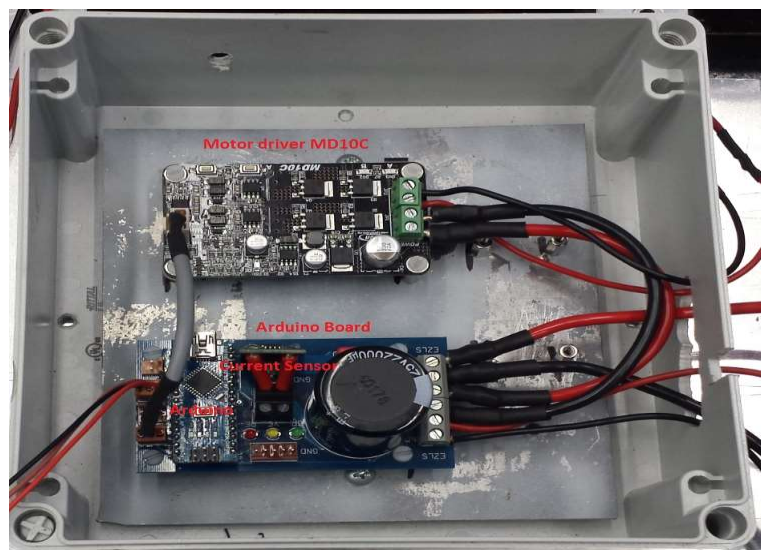
Figure 3.16 Motor Driver MD10C with Arduino Board and current sensor
