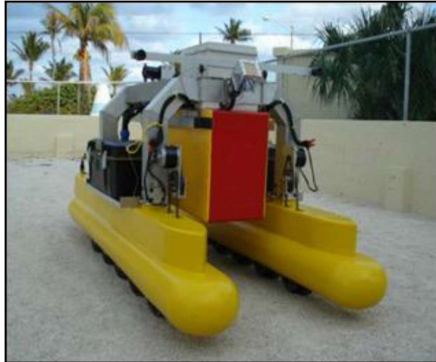
Figure 1.10 The DUKW-Ling Unmanned Amphibious Vehicle
