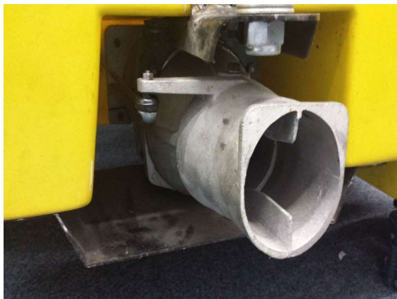
Figure 8.4 Water jet steering box
