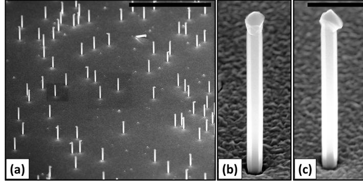
Figure A.2: (a) SEM image of the NW ensemble on sample 2 where the NW density is  $1/\mu\text{m}^2$ . (b) and (c) demonstrate the smooth morphology of two randomly selected single NWs. Scale bars in (a) and (c) are  $20\ \mu\text{m}$  and  $1\ \mu\text{m}$ , respectively. (b) and (c) have the same scale.
