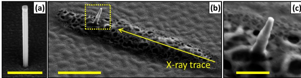
Figure C.3: (a) SEM micrograph of NW12 before exposure. (b) NW 12 after exposure. The yellow arrow indicates the trace of the X-ray beam on the substrate. (c) Zoom in of the area marked by a yellow box in (b).
