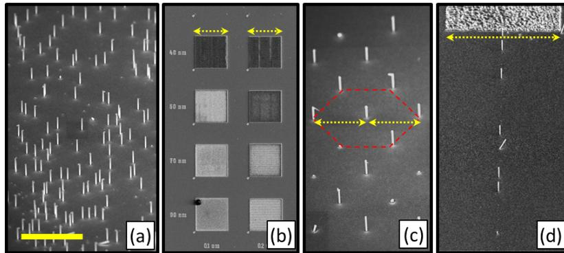
Figure 2.6: (a) NW growth on native oxide Si 111 substrate. (b) SAG quadratic NW fields. (c) SAG NW growth with hexagonal pattern, marked by a red dotted hexagon. (d) selective NW growth along a straight line. The scale bar in (a) and the arrows in (b,c,d) are 15, 100, 10 and 50  $\mu\text{m}$ , respectively.
