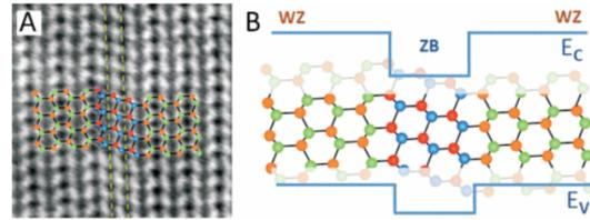
Figure 2.4: (a) HAADF HRSTEM micrograph of a ZB quantum well in a WZ segment. (b) An atomistic model of a WZ/ZB/WZ heterostructure along with a schematics of the band diagram [97].
