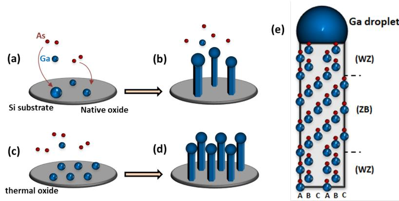
Figure 2.5: Animations (a,b) and (c,d) illustrate the NW growth procedure on Si substrates with native and thermal oxide layers using the self-assisted VLS growth mechanism, respectively. (e) Side view scheme of a NW composed of WZ and ZB polytypes.
