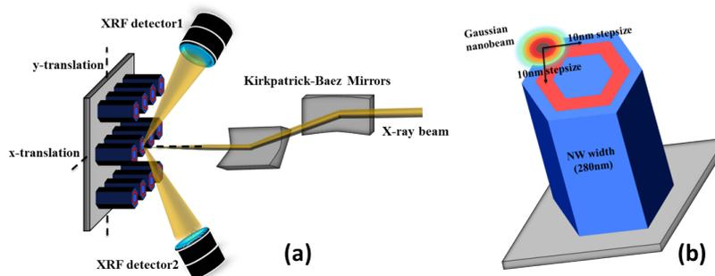
Figure 4.4: (a) A schematic illustration of the setup at the XRF station ID16b of the European Synchrotron Radiation Facility. (b) Sketch of how the X-ray nanobeam is scanned across the NW area during the XRF experiment.
