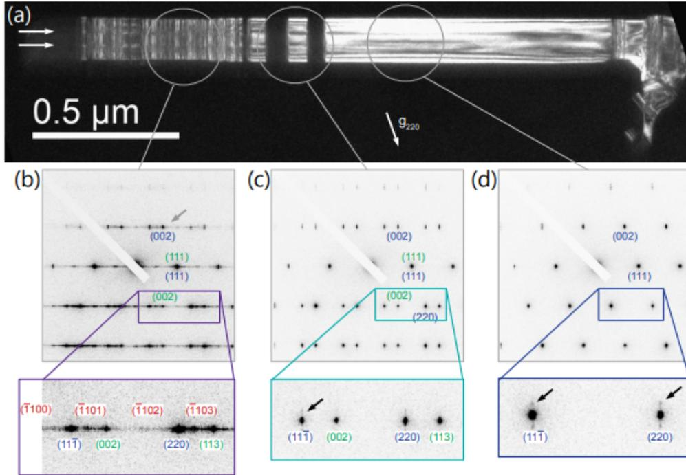
Figure 6.4: (a) Transmission electron micrograph taken in dark-field mode on a core-shell NW. The three panels in (b), (c), and (d) show electron diffraction measurements at different positions of the NW. Here, the labels indicate the respective lattice vector in reciprocal space and the arrows indicate diffraction spots suggesting a coherently strained shell.
