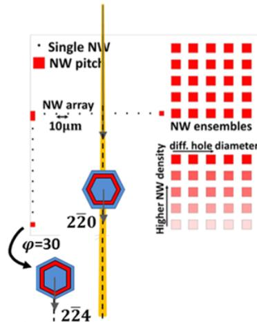
Figure B.1: Top view of the lithography patterned sample mask along the NW orientation when the incident beam is perpendicular to the NW array. Single dots represent positions of single NWs.
