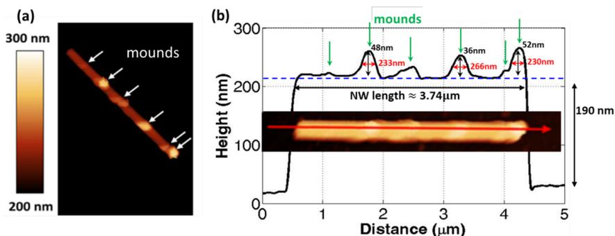
Figure 4.10: (a) Atomic force microscopy image of a dispersed NW from sample 3. (b) Line profile along the NW axis.
