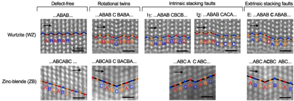
Figure 2.3: TEM images showing stacking sequences of WZ and ZB including rotational twins and stacking faults in InAs and InAsASb NWs.
