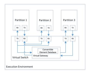
FIGURE 5.16: General Architecture of the Virtual Gateway
