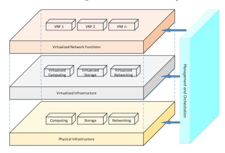
FIGURE 3.4: Network Function Virtualization Architecture
