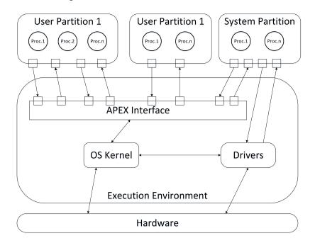
FIGURE 3.1: ARINC 653 System Architecture
