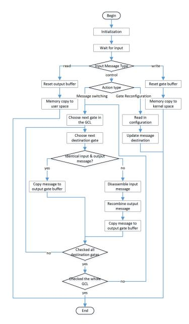
FIGURE 5.20: Workflow of the Data Plane
