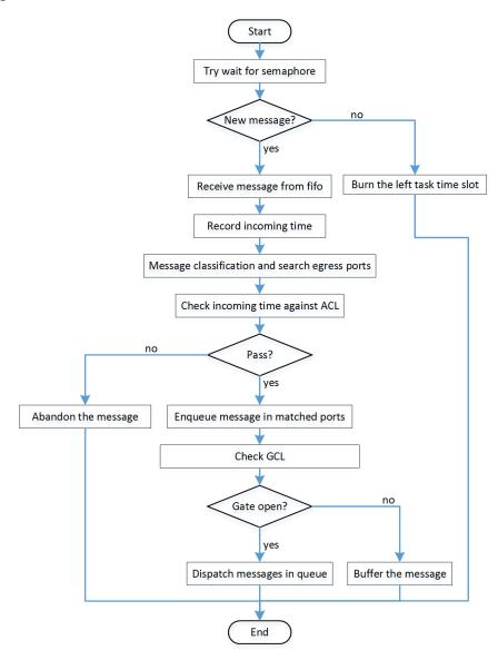
FIGURE 5.29: Workflow of Virtual Switch
