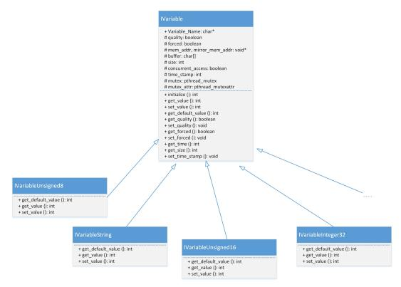
FIGURE 4.11: Structural Design of Variable Manager
