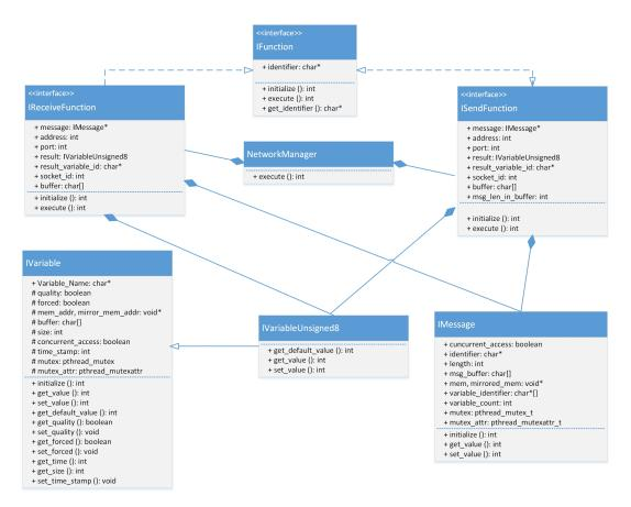
FIGURE 4.13: Structural Design of Network Manager
