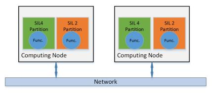
FIGURE 2.4: Example of Mixed-Criticality Architecture
