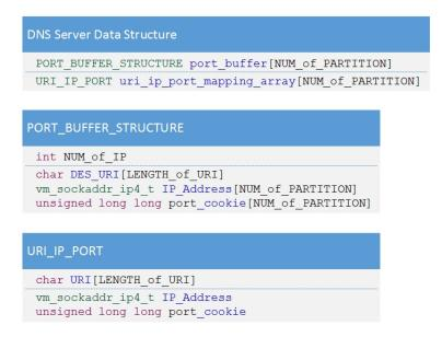
FIGURE 5.7: The Major Data Structure in DNS Server
