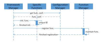
FIGURE 4.6: Function Initialization Procedure
