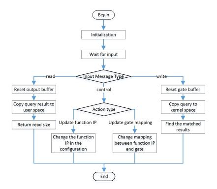
FIGURE 5.21: Workflow of the DNS Server
