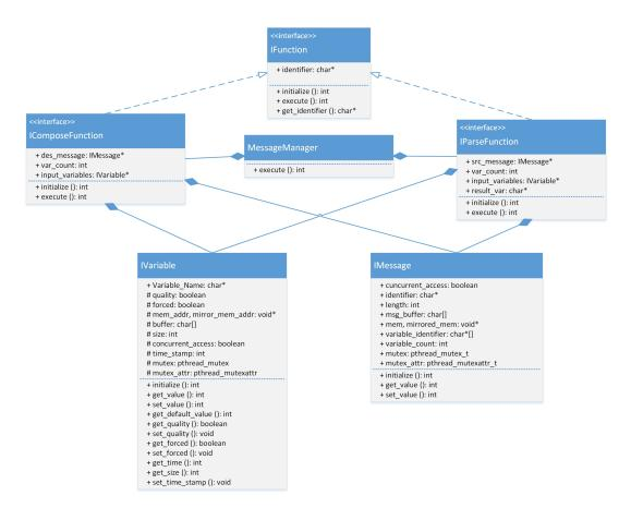
FIGURE 4.12: Structural Design of Message Manager
