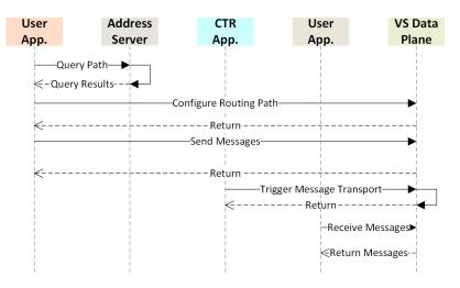
FIGURE 5.4: Data Communication Process
