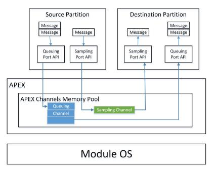
underlying channels. A channel is the logical link between partitions and statically configured during system integration.
