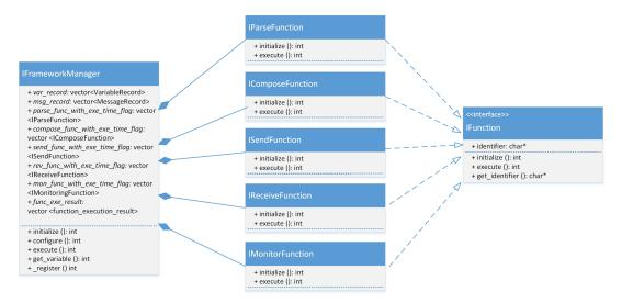
FIGURE 4.8: Structural Design of Framework Manager
