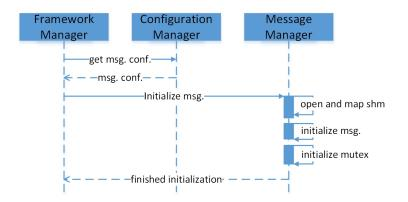
FIGURE 4.5: Message Initialization Procedure
