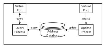
FIGURE 5.3: Architecture Model of VS Address Server
