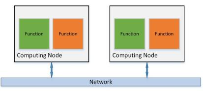
FIGURE 2.3: Example of an Integrated Architecture
