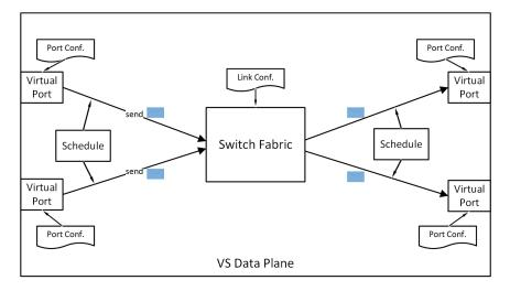
FIGURE 5.2: Architecture Model of VS Data Plane
