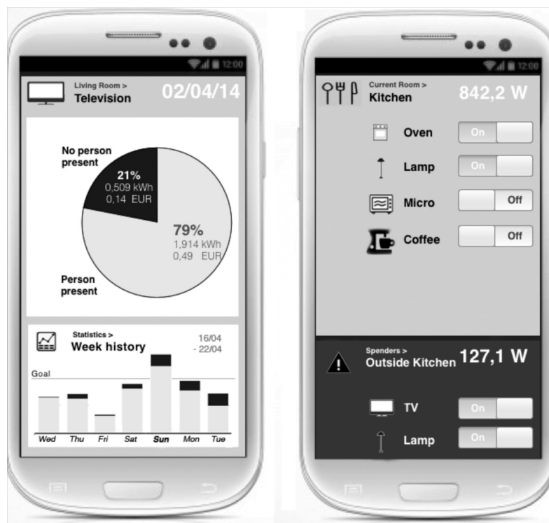
Figure 24. Using room-context information to enrich eco-feedback visualization (left) and to adapt home control interfaces (right)
