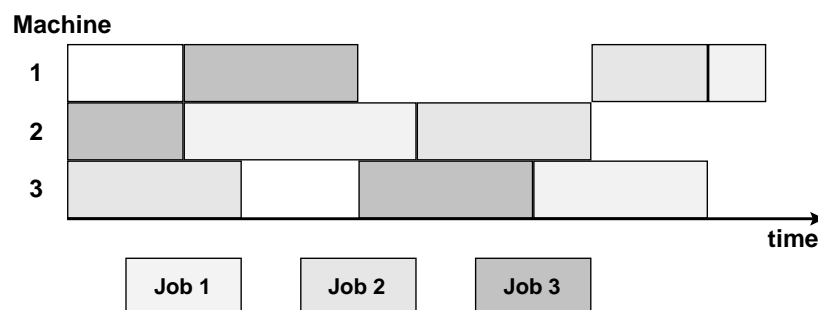
Figure 2.4: A solution to a 3-jobs/3-machines instance of the JSSP
