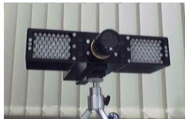
Figure 3.9: A photograph of the 48 x 64 pixel PMD camera.
