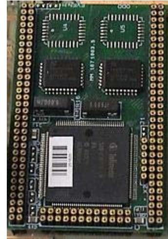
Figure A.1: Infineon Minimodule C167 CR-LM
