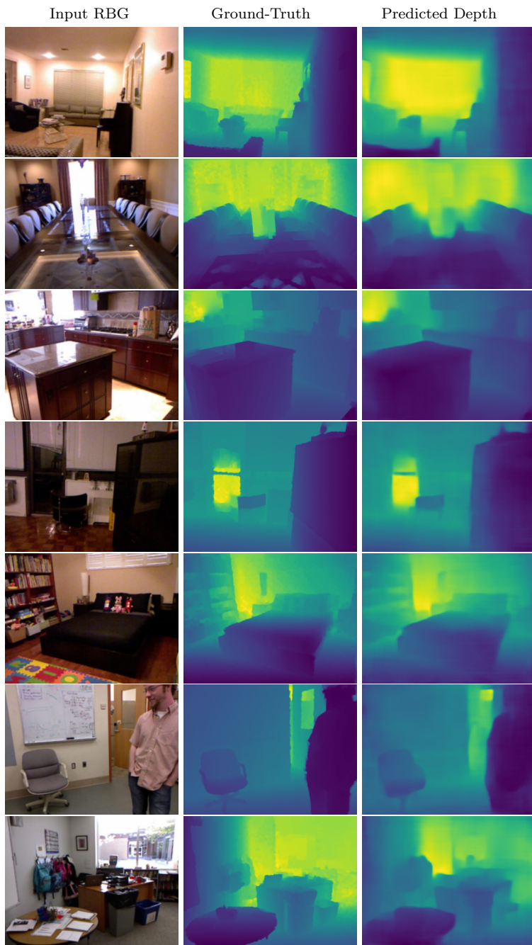
Figure 4. Output of our model on NYU RGB-D dataset. The first row shows the input RGB image, the second row shows the ground truth depth image, and the last row shows the estimated depth image of our method.
