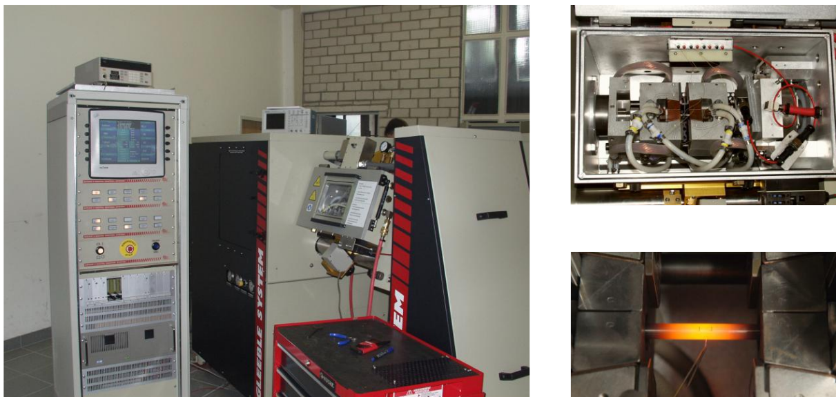
Figure 3-4: Forming dilatometer type Gleeble© 3500.
