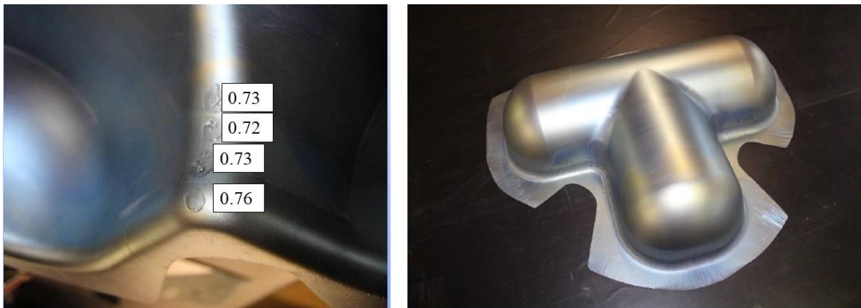
Figure 4-38: Thickness of the critical curve of half-shell manufactured by FormTech ® according to suggested parameters.
