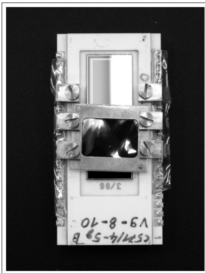
Figure 4.7: The XMM-type pnCCD with the mesh mounted directly on the ceramic board.
