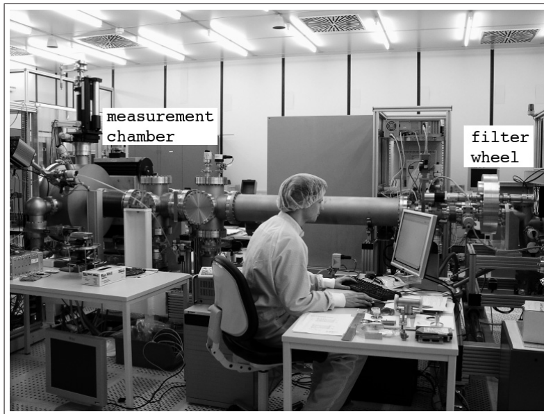
Figure 4.2: A view of the Röstli test facility. The X-ray tube not visible here has various anode targets mounted on a wheel which can be operated from outside the vacuum. During measurements and when the pnCCD is cooled, the evacuated volume is kept at pressures below 1.0 \cdot 10^{-6} mbar. At higher pressures, residual gases could condense on the entrance window and affect the device performance by absorbing low energy X-rays.
