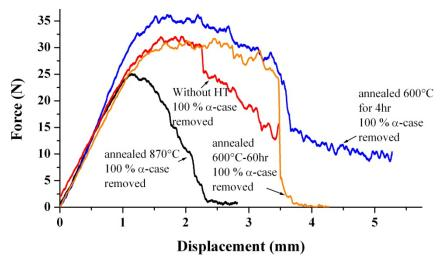
Figure 4.19: Uniaxial-bending test of heat-treated and acid-cleaned samples
