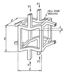
Figure 2.28: Linear elastic strut bending of an open-cell foam model [3]
