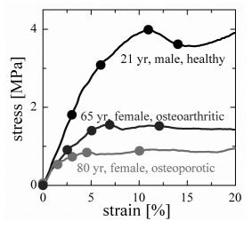
Figure 2.6: Effect of osteoarthritis, and osteoporosis in the compressive strain-stress curve of a trabecular human cuboid bone [91]
