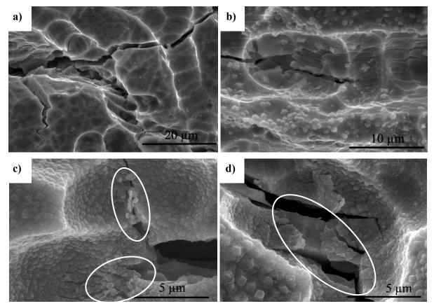
Figure 4.29: Micrograph of the coated samples after the cyclic bending test: a) SBI, b) SBII, c) SBIII and d) SBIV
