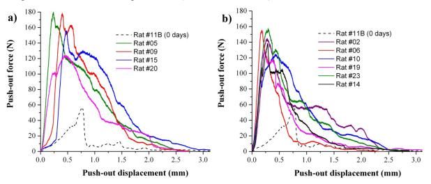
Figure 4.32: Push-out behaviour of the a) coated rat implants, b) uncoated rat implants
