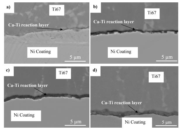
Figure 4.25: Cross-sectional micrograph of the Ca-Ti reaction layer: a) SBI, b) SBII, c) SBIII and d) SBIV
