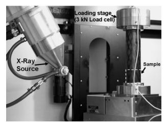
Figure 3.14: µCT system with loading stage
