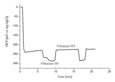
Figure 5.1: Open circuit potential of Ti67 submerged in the HNO<sub>3</sub>+ HF bath
