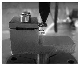
Figure 3.10: Monotonic bending system for grid-shaped samples
