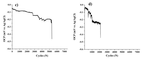
Figure 4.28: OCP curves of the coated samples: a) SBI, b) SBII, c) SBIII and d) SBIV
