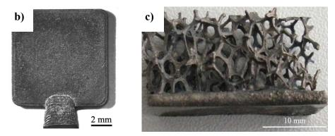
Figure 3.7: a) Grid-shaped specimen, b) plate sample and c) cast Ti67 sponge
