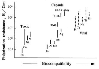
Figure 2.9: Relationship between polarization resistance and biocompatibility of pure metals, Co-Cr alloy and stainless steels [122]
