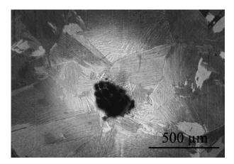
Figure 2.21: Ceramic shell inclusions in titanium investment casting [200]
