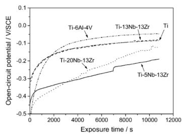
Figure 2.11: Variation of OCP with exposure time for CP-Ti, Ti-6Al-4V, and Ti-xNb-13Zr alloys in Ringer's solution at 37°C [143]
