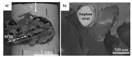
Figure 4.41: SEM micrograph of the ovine implants after the push-out test: a) external surface of the implant of the sheep #2, b) surface at the internal implant strut of the sheep #22
