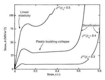
Figure 2.4: Compressive stress-strain curve of cancellous bone for different relative densities of wet trabecular bone [3]
