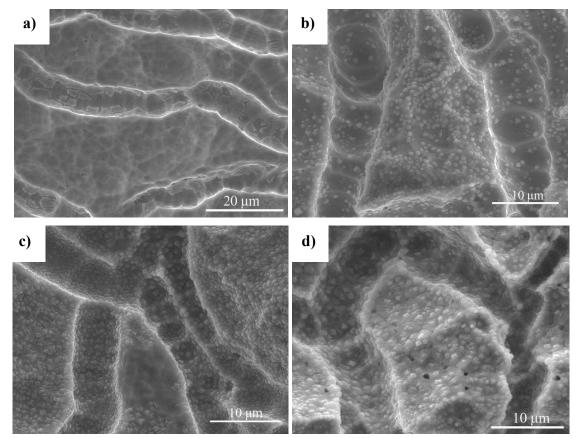
Figure 4.24: Sample surfaces coated with: a) SBI, b) SBII, c) SBIII and d) SBIV
