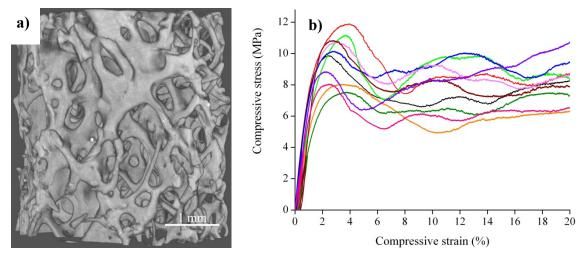
Figure 4.2: Bovine cancellous bone: a) 3D reconstruction of a part of the bone used for the compression test, b) compression behaviour of the cancellous bone
