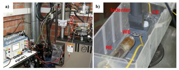
Figure 3.11: a) Corrosion system used in the cyclic bending, b) detail of the corrosion-testing chamber
