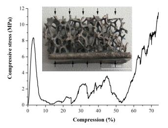
Figure 4.15: Stress vs. compression curve of Ti67 sponge
