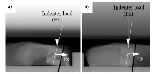
Figure 5.4: Eliminated force components during the push-out test: a) longitudinal force Fx and b) lateral force Fy
