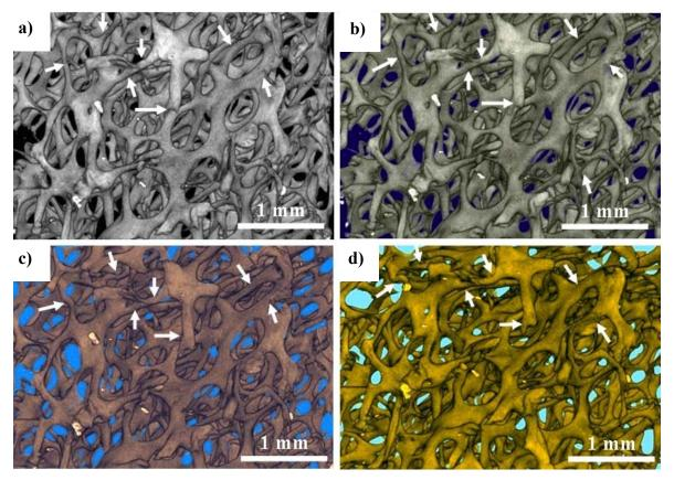
Figure 4.4: µCT-analysis of the deformation occurring during step-wise compression of the bovine cancellous bone: a) at 0% stress, b) at yield, c) at maximum stress, d) plastically deformed
