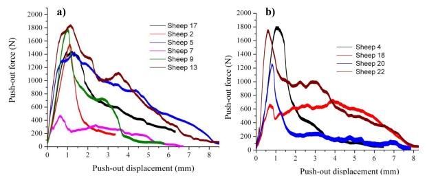
Figure 4.38: Push-out behaviour of the a) coated ovine implants, b) uncoated ovine implants
