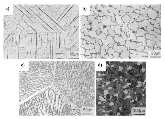
Figure 2.15: a) Acicular martensite in Ti-6Al-4V quenched from  $\beta$  phase field, b) fully equiaxed microstructure of a Ti-6242, c) lamellar  $\alpha + \beta$  microstructure in Ti-6Al-4V slowly cooled from the  $\beta$  phase field, d) Bi-modal microstructure of a IMI 834 [9]
