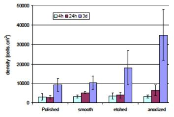
Figure 2.13: Cell density on polished, smooth, etched and anodized surfaces of titanium implants, after 4 hours, 24 hours, 3 days [152]
