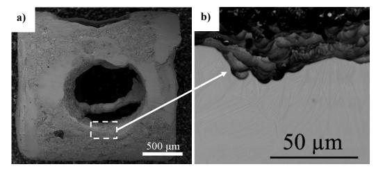
Figure 4.20: a) Pickled rat implant, b) surface details of the implant at the border of the implants holes
