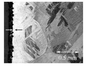
Figure 2.20: Micrograph of a cast Ti sample: arrows show the  $\alpha$ -case thickness [190]
