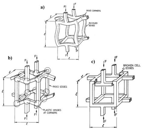
Figure 2.29: Dimensional analysis of cell collapse in an open-cell foam by a) buckling, b) plastic yielding and c) brittle fracture [3]
