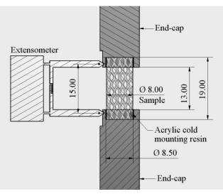
Figure 3.13: Schematic of the experimental set-up
