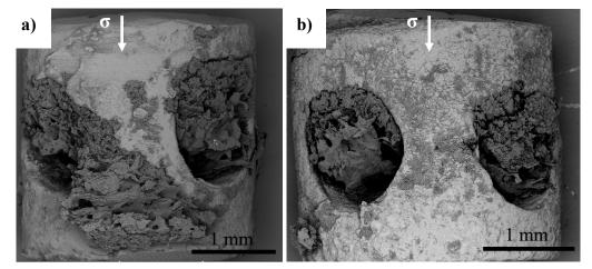
Figure 4.33: SEM micrograph of the rat implants after push-out test: a) coated implant, b) uncoated implant
