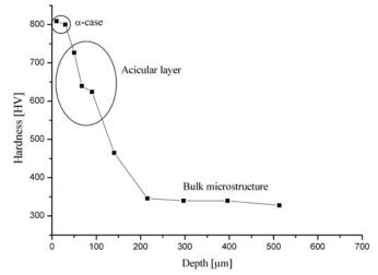
Figure 4.11: Vickers microhardness vs. distance from the surface in a cast Ti67 specimen
