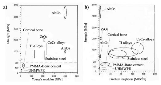
Figure 2.7: Comparison of the mechanical properties of different biomaterials used in orthopaedic implants: a) strength vs. Young's modulus and b) strength vs. fracture toughness [103]
