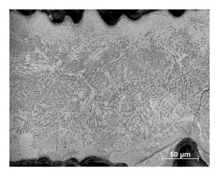
Figure 4.17: Cross section microstructure of a grid-shaped sample after annealing at 1060°C for 1 hr
