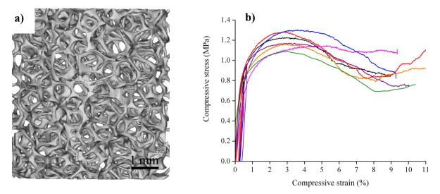
Figure 4.5: 45ppi open-cell AlSi7Mg foam: a) 3D reconstruction of a sample used for the compression test, b) compression behaviour of the foam
