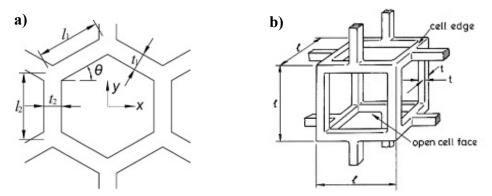
Figure 2.27: a) Honeycomb cell model, b) 3-D model of an open-cell foam [3]
