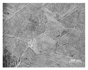
Figure 4.18: Microstructure of a cast Ti67 sample aged at 600°C for 4 hr
