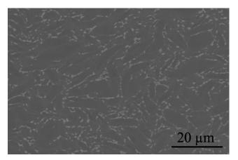
Figure 3.5: Globular microstructure of rolled Ti-6Al-7Nb ingot
