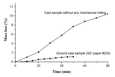
Figure 4.21: Gravimetric measurements of the mass loss during pickling of cast Ti67 samples without any prior mechanical milling and cast Ti67 samples ground with an abrasive paper
