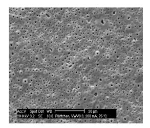
Figure 2.12: Titanium implant with porous coating based on calcium phosphate[148]
