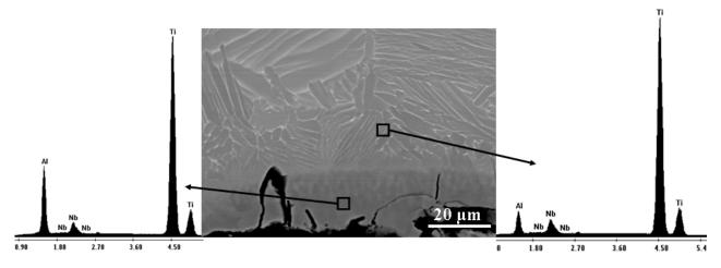
Figure 4.9: SEM micrograph with two EDS spot analyses of the chemical composition of the  $\alpha$ -case and the coarse acicular zone, respectively, revealing the high Al concentration in the outermost zone
