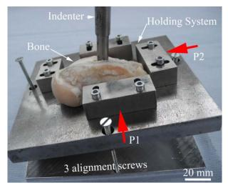
Figure 3.18: Push-out testing system used to analyse the ovine bone-implant interface (P1 and P2 are the directions used for the X-ray analysis)
