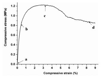
Figure 4.6: Mechanical response of the 45ppi open-cell AlSi7Mg foam with the four deformation points tested in the in-situ loading stage
