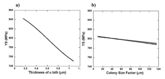
Figure 2.18: Variation of the yield strength of a Ti67 alloy with: a) the thickness of the lath and with the b) colony scale factor [186]
