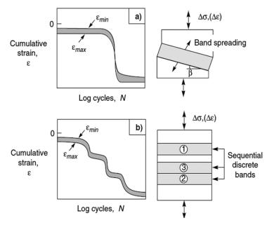
Figure 2.31: Typical behaviours in compression-compression fatigue of metallic foams at a fixed stress range: a) Progressive shortening by broadening of a single crush band with increasing cycles, b) sequential formation of crush bands [224]
