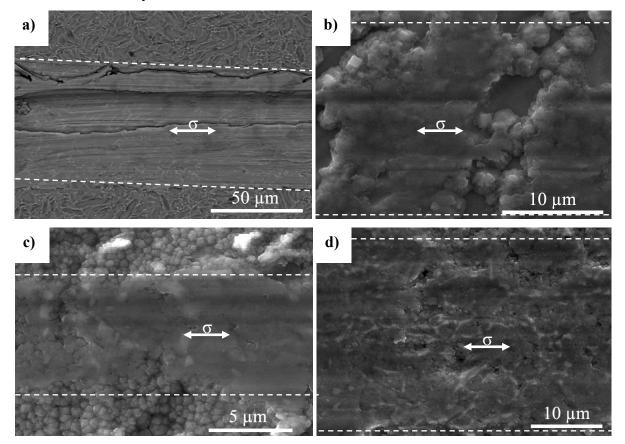
Figure 4.30: SEM micrograph of the coatings after the friction test: a) SBI, b) SBII, c) SBIII, d) SBIV
