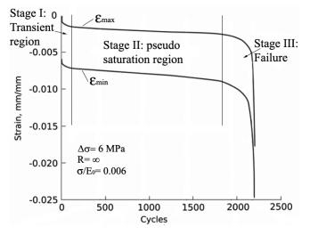
Figure 2.5: Strain evolution as a function of numbers of cycles of bovine cancellous bone [79]
