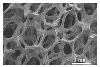
Figure 3.9: Structure of 45ppi open-cell AlSi7Mg foam
