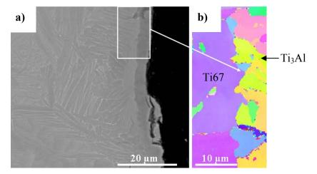
Figure 4.10: a) SEM micrograph of a cast Ti67sample and b) corresponding EBSD orientation mapping of the interface between the fine grained  $\alpha$ -case layer and the coarse acicular  $\alpha+\beta$  Ti structure
