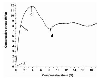
Figure 4.3: Mechanical response of the bovine trabecular bone with the four deformation points tested in the in-situ loading stage
