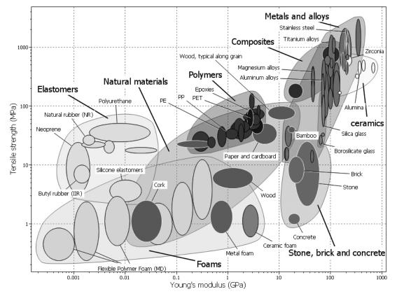
Figure 2.22: Young modulus vs. tensile strength of engineering materials [3]
