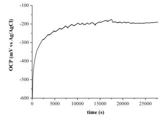
Figure 4.26: Open-circuit potential of a cast Ti67 uncoated sample
