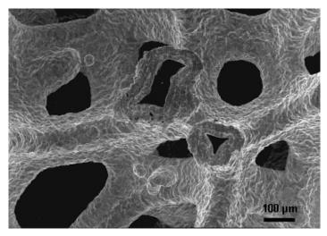
Figure 2.24: SEM micrograph of a tantalum foam [221]
