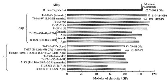
Figure 2.16: Elastic modulus of various Ti- alloys used as biomaterials [174]
