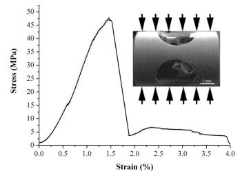
Figure 4.23: Compression behaviour of an ovine implant
