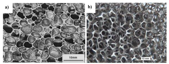
Figure 2.23: a) closed-cell foam [210], b) open-cell foam
