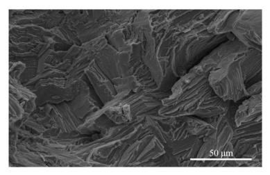
Figure 4.16: SEM micrograph of the fracture surface of a Ti67 sponge after compression testing
