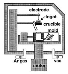
Figure 2.17: Schematic representation of the centrifugal titanium casting machine [180]
