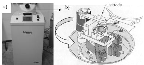
Figure 3.6: a) Centrifugal casting machine, b) schematic of the casting chamber
