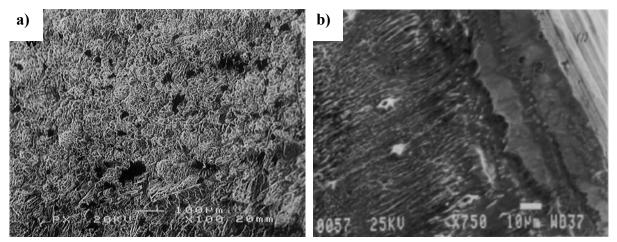
Figure 2.10: a) Pitting corrosion in a welded REX 734 stainless-steel orthopaedic implant [136],
