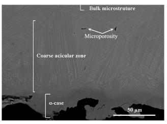
Figure 4.8: SEM micrograph of a Ti67 cast sample
