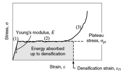
Figure 2.26: Schematic representation of the compression strain-stress curve of a metallic foam [224]
