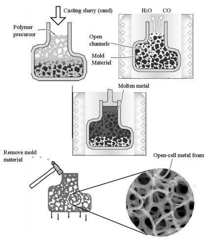
Figure 2.25: Investment casting method used to manufacture open-cell foams [224]
