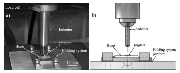
Figure 3.17: Push-out testing system used to analyse the bone-implant interface a) push-out system used for the rats, b) Frontal schematic of the push-out test
