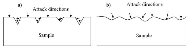
Figure 5.2: Schematic representation of the effective surface for acid attack with a) pitting corrosion marks and b) worm marks
