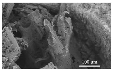
Figure 4.35: SEM micrograph of a failed trabeculae located in the holes of the implants
