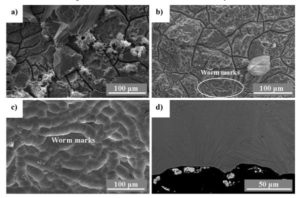
Figure 4.14: Pitting corrosion after: a) 20 min, b) 40 min, c) 60-70 min of pickling, and d) cross sectional SEM micrograph after 60-70 min of pickling
