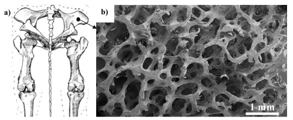
Figure 3.4: a) Position of the extracted bovine bone samples (modified from [245], b) SEM micrograph of cancellous bovine bones at the iliac crest
