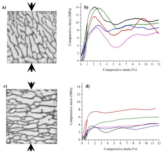
Figure 4.1: Ovine cancellous bone: a) orientation of the trabeculae along the MTD, b) compression behaviour along the MTD, c) orientation of the trabeculae perpendicular to the MTD, d) compression behaviour perpendicular to the MTD
