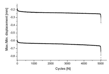
Figure 4.27: Cyclic displacement behaviour of a sample coated with SBIII
