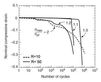
Figure 2.30: Progressive shortening behaviour in compression-compression fatigue for a Duocel Al-6101-T6 foam of relative density 0.08 [224]
