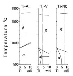
Figure 2.14: Section of phase diagrams of binary titanium systems: Ti-Al, Ti-V and Ti-Nb [164]
