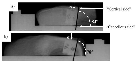
Figure 4.37: Example of the inclination angle of the ovine implant: a) lateral position, b) front position of the push-out system
