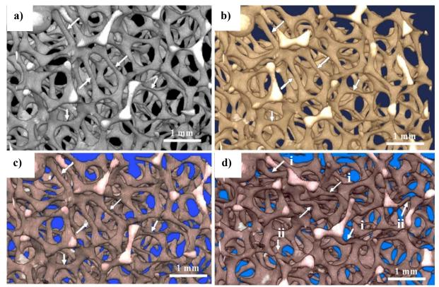
Figure 4.7: µCT-analysis of the deformation occurring during step-wise compression of the 45ppi AlSi7Mg foam: a) at 0% stress, b) at yield, c) at maximum stress, d) plastically deformed
