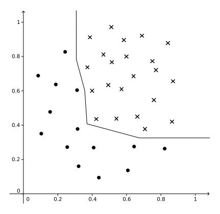
Figure 2.4: Example of a not linearly separable problem: separating dots from crosses.
