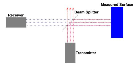
Figure 5.13: Optical paths united by a beam splitter.
