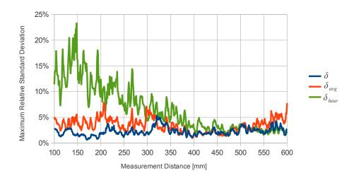
Figure 7.14: Maximum relative deviation  $\delta$  computed from  $\vec{r}$  with  $\rho = 8$  mm for the presented methods on set  $T_2$ .
