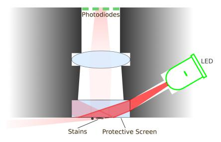
Figure 5.20: Detecting dust using an additional LED.
