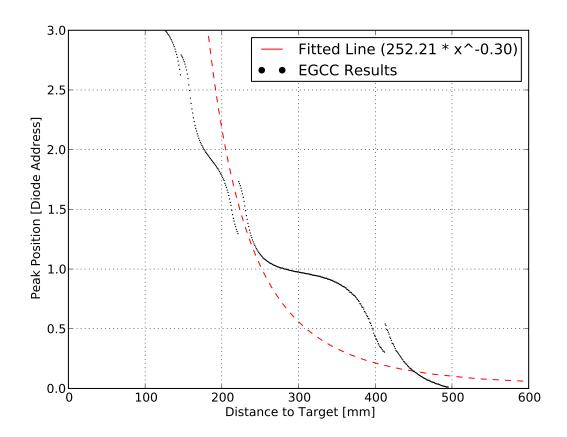
Figure 2.7: Power-function model on EGCC-results vs. true measurement distance (see [4]).
