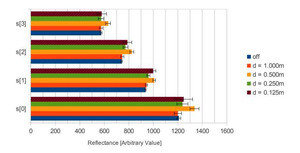
Figure 7.26: Averaged spectral signatures with standard deviation acquired at different positions of a DC powered 50 W lamp.
