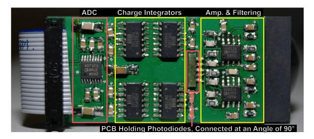
Figure 5.26: Photocurrent readout PCB.
