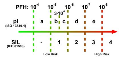
Figure 5.12: Classification of risks by ISO 13849-1 and IEC 61508 [46, Tab. 4] [47, Tab. 3].
