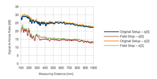
Figure 7.23: Signal-to-noise ratios of  $\vec{s}[0]$  and  $\vec{s}[2]$  from measurements of the wooden board. Acquired with and without field stop.
