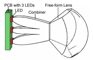
Figure 3.2: Free-form lens to combine three LEDs. Original source: [31, Fig. 3].
