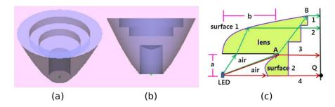
Figure 3.3: Illustration of a free-form lens. The lens is depicted in an isometric view (a), a right view (b) as well as a sectional drawing for half a lens including exemplified ray paths (c). Source: [33, Fig. 2+3].
