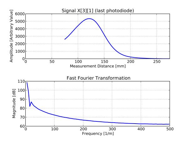
Figure 7.3: FFT of a signal from the last photodiode.
