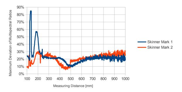
Figure 7.20: Maximum deviation of ratios within spectral signatures acquired at partial beam coverage to a wooden board using Skinner mark 1 and mark 2 sensors.
