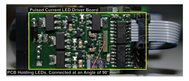
Figure 5.25: LED driver to generate pulses at controlled current.
