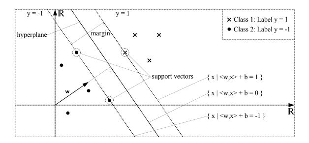
Figure 2.3: Linear separation of two classes by a hyperplane in a two-dimensional example [12, see Fig. 1.5].
