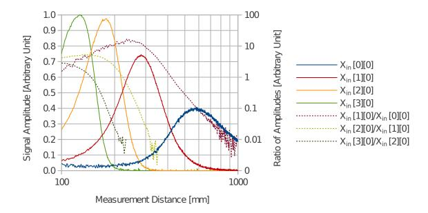
Figure 6.6: Sensor readings combined with ratios of signals from neighboring photodiodes on a logarithmic scale.
