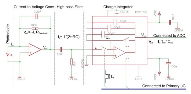
Figure 5.27: Schematic of the circuit for a single photodiode.
