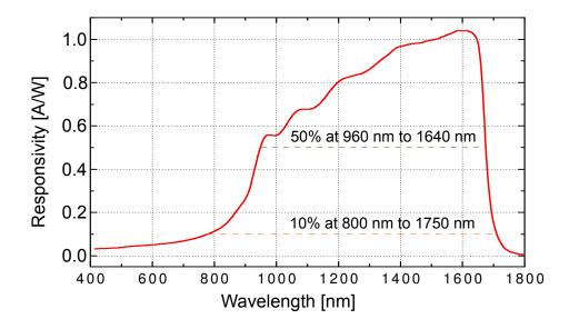
Figure 5.5: Spectral responsivity of an InGaAs photodiode (Original source: [60]).
