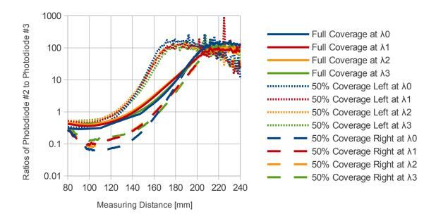
Figure 7.19: Signal ratio of neighboring photodiodes. Measured at full and partial beam coverage using a Skinner mark 1 sensor.
