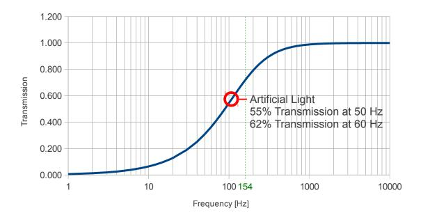
Figure 6.2: Transmission characteristic of the used  $f_c$  = 154Hz high-pass filter of first order.
