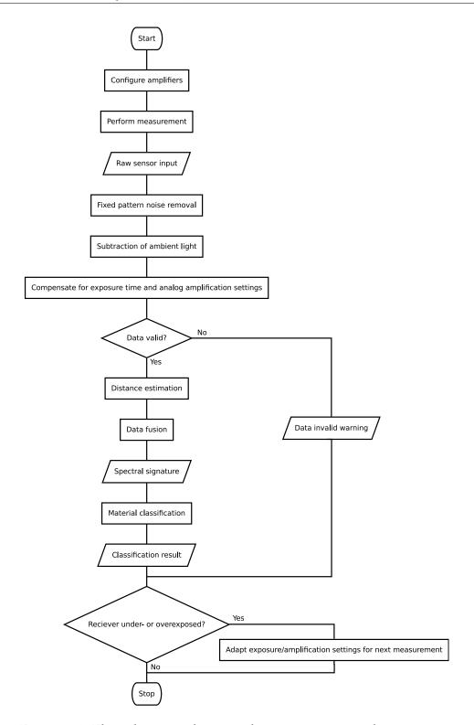
Figure 6.1: Flow diagram showing data acquisition and processing.
