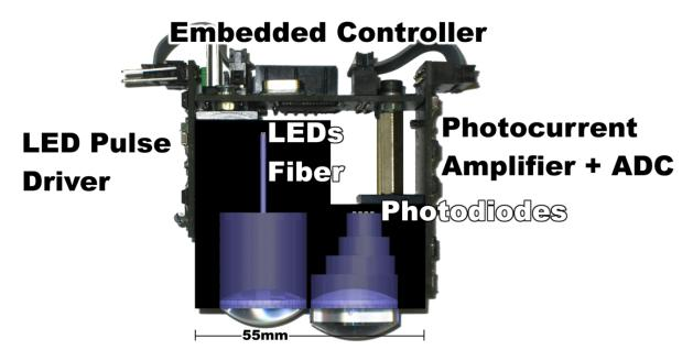
Figure 5.22: Virtually augmented photograph of the implemented sensor. Source: [5, Fig. 3].
