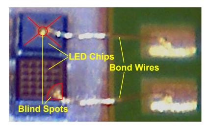
Figure 5.17: Image of two LED chips with bond wires.
