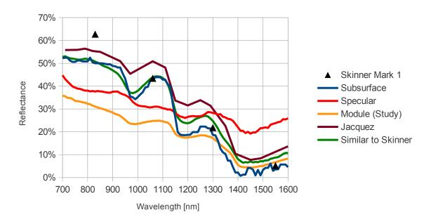
Figure 4.10: Subsurface and specular reflectance components in comparison to measurements performed with the measurement setup used for the study, a spectroscopy setup which is similar to the Skinner sensor and data by Jacquez et al. [9].
