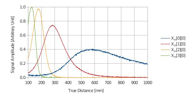
Figure 6.5: Sensor readings of all four photodiodes acquired at  $\lambda_0 = 830 \,\text{nm} \, (\mathbf{X}_{in}[0][0]$  to  $\mathbf{X}_{in}[3][0]$ ).
