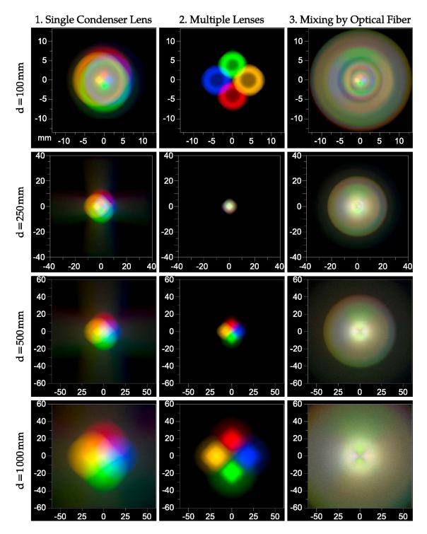
Figure 5.19: False color images of simulated projections from three concepts at four projection distances. All units in millimeter. Note that the scale changes with projection distance.
