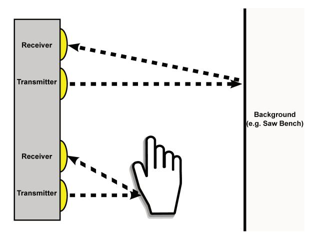
Figure 5.7: Single-sided multispectral barrier configuration.
