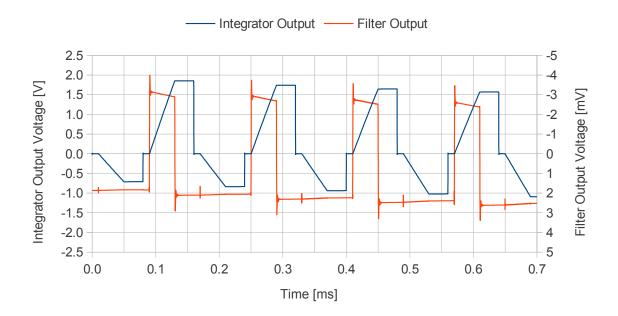
Figure 6.4: Simulation of high-pass filter and integrator output.
