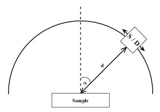
Figure 4.7: Measurement setup for angular dependent reflectance measurement comprising light source S, light detector D, angle of incidence  $\alpha$  and the distance of measurement d [42, Fig. 4.2].
