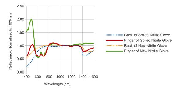
Figure 8.5: Reflectance spectra of new and soiled nitrile gloves, normalized to the reflectance at 1070 nm.
