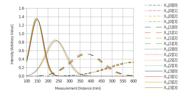
Figure 7.7: Gaussian functions as noise free synthetic sensor data  $(T_4)$ .
