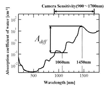
Figure 3.1: Absorption coefficient of water in the visual and near-infrared spectrum (Source: [27, Fig. 4]).
