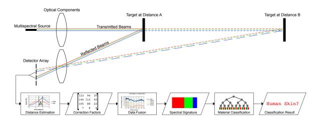
Figure 1.1: Principle setup and signal processing of a multispectral point sensor for material classification (compare [4, Fig. 1]).
