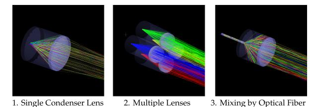
Figure 5.18: Overview of beamforming concepts.
