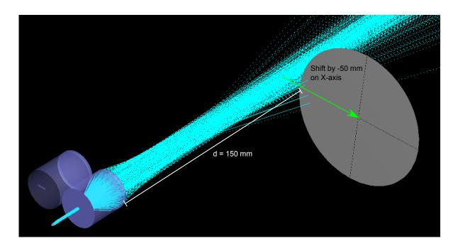
Figure 7.4: Simulation of sensor (M1) showing target shifted by -50 mm at d = 150 mm. all methods perform very poor on the shifts by  $\pm 50$  mm, where the overlap of object and beam is minimal, especially for short measurement distances (see Fig. 7.4).
