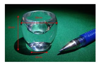
Figure 3.4: The prototype of the collimator lens by Chen et al.. Source: [34, Fig. 11].
