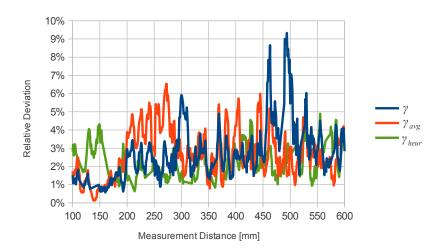
Figure 7.10: Relative deviations with  $\rho = 8$  mm for the presented methods on set  $T_3$ .
