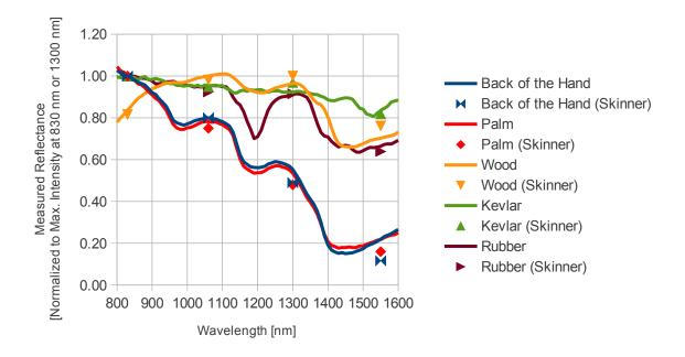
Figure 4.3: Mapping of reflectance measurements acquired using the *irSys*®1.7 spectrometer to measurements of the Skinner mark 1 sensor system.
