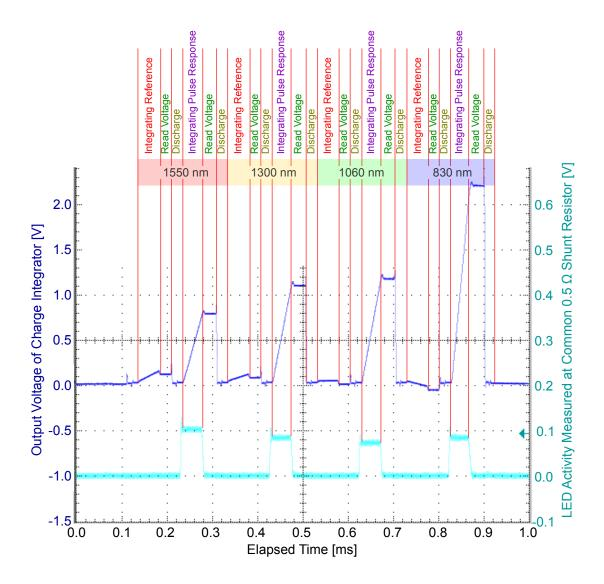
Figure 6.3: Output signal of a charge integrator during signal acquisition.
