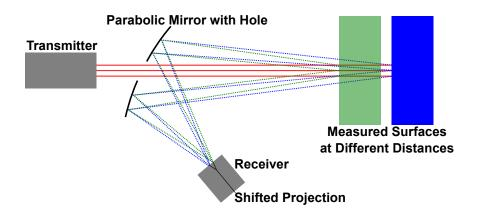
Figure 5.14: Optical paths aligned using a parabolic mirror. Distance dependent projections are illustrated.
