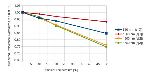
Figure 7.28: Spectral signatures acquired from 0 °C to 50 °C using a Skinner mark 2 sensor.
