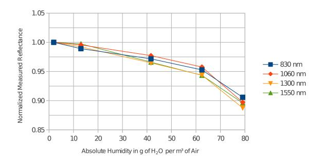
Figure 7.27: Atmospheric attenuation measured using a Skinner mark 2 sensor.
