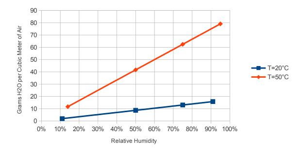
Figure 5.2: Mapping of temperature and relative humidity to absolute humidity.
