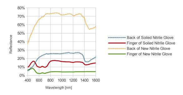
Figure 8.4: Reflectance spectra of new and soiled nitrile gloves.
