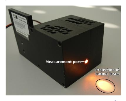
Figure 4.4: Reflectance measurement module for *irSys*®1.7.
