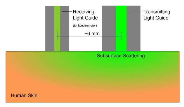
Figure 4.8: Setup to measure the subsurface components of the reflection spectrum.
