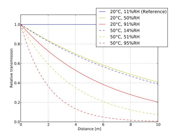
Figure 5.4: Relative transmission at 1365 nm.
