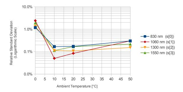
Figure 7.29: Relative standard deviation of spectral signatures acquired over a temperature range from 0 °C to 50 °C.
