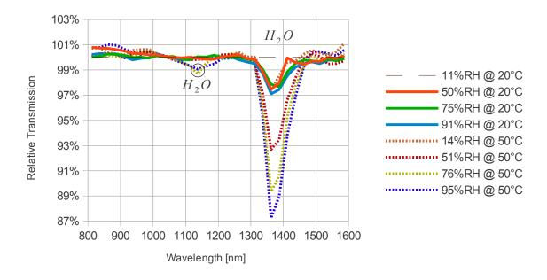
Figure 5.3: Relative transmission over an air path length of 0.34 m. The reference measurement was acquired at a temperature of 20 °C and 11 % RH.
