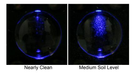
Figure 5.21: Sideways illuminated protective screen showing very low and medium soil level.
