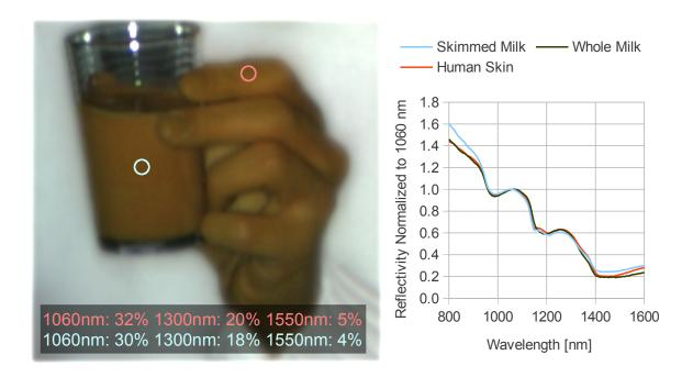
Figure 5.8: False color image and plot of skimmed and whole milk as well as human skin. False color mapping:  $1060 \,\text{nm} \mapsto \text{red}$ ,  $1300 \,\text{nm} \mapsto \text{green}$  and  $1550 \,\text{nm} \mapsto \text{blue}$ .
