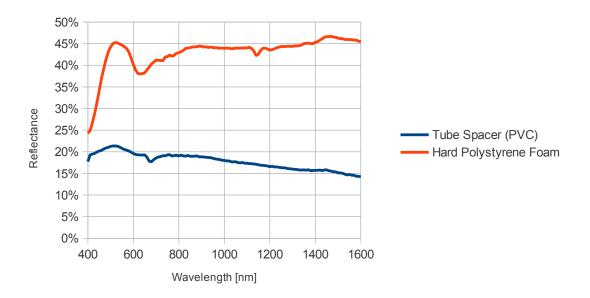
Figure 8.6: Reflectance spectra of common workpieces at construction sites.
