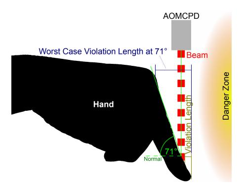
Figure 5.9: Illustration of a finger passing the beam at an acute angle.
