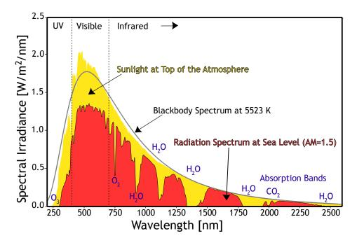
Figure 5.1: Atmospheric attenuation - a comparison of irradiance at sea level and the top of the atmosphere (Source: [54]).
