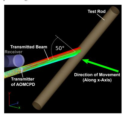
Figure 5.10: Test rod at acute angle to transmitted beam.
