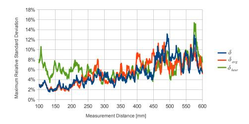
Figure 7.15: Maximum relative deviation  $\delta$  computed from  $\vec{r}$  with  $\rho = 8$  mm for the presented methods on set  $T_3$ .
