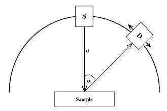
Figure 4.5: Measurement setup for scattering measurement comprising light source S, light detector D, angle of incidence  $\alpha$  and the distance of measurement d [42, Fig. 4.1].
