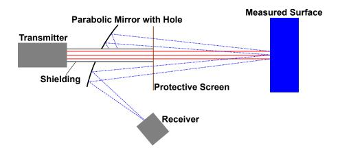
Figure 5.15: Optical paths aligned using a parabolic mirror. Obstruction by additional shielding is illustrated.
