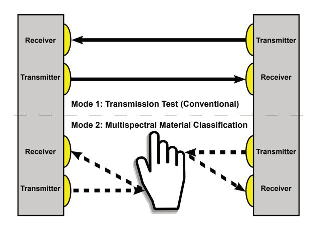
Figure 5.6: Two-sided multispectral light curtain configuration.
