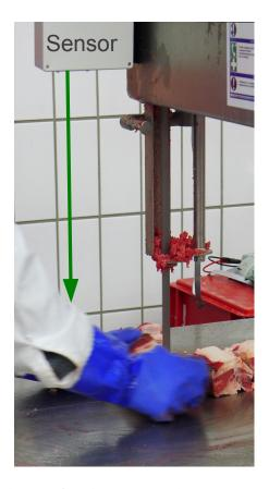
Figure 8.2: Practical test of a Skinner mark 2 sensor at a bone band saw.
