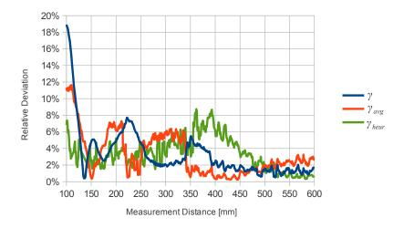
Figure 7.8: Relative deviations with  $\rho = 8$  mm for the presented methods on set  $T_1$ .
