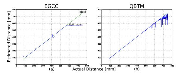
Figure 7.5: Distance estimation from 100 mm to 800 mm on actual sensor data using EGCC and QBTM (Compare [4, Fig. 10]).
