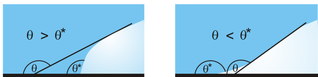
Figure 2.3. On the nanoscale, the shape of bubbles may deviate from a spherical cap and the contact angle may be over- or underestimated.
