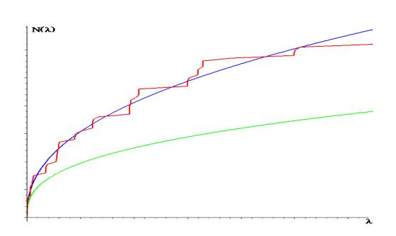
Figure 5.6:  $N(\lambda)$  as a function of  $\lambda$  for the fifth order measure geometric beaded string with scaling ratios  $r_1 = \frac{1}{4}$  and  $r_2 = \frac{1}{3}$ , blue: power-law fit, green: expectation from Equation 5.3.
