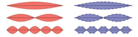
Figure 3.2: Corresponding vibrational modes of a string and a monoatomic chain
